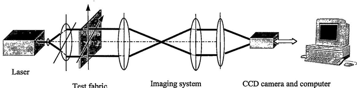
**Figure 5.1 : Optoelectronics system for defect detection by Rank order filtering method**
