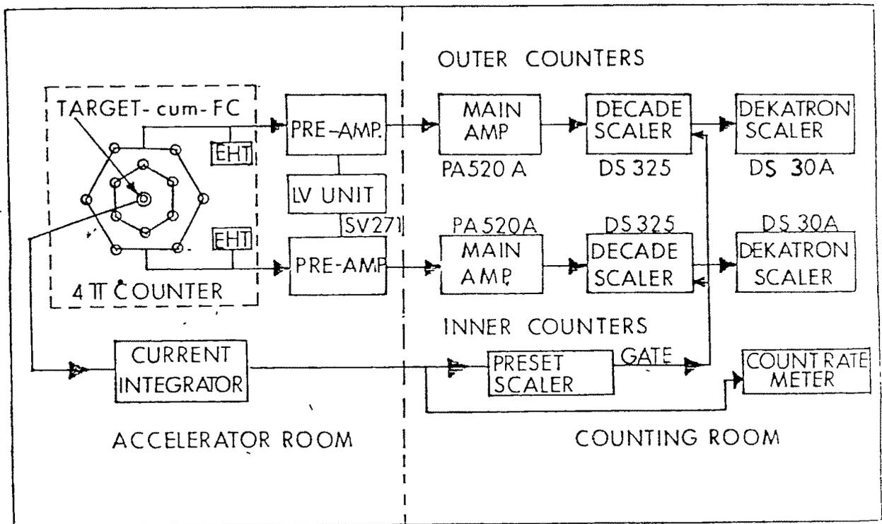
(b) BLOCK DIAGRAM OF ELECTRONICS
