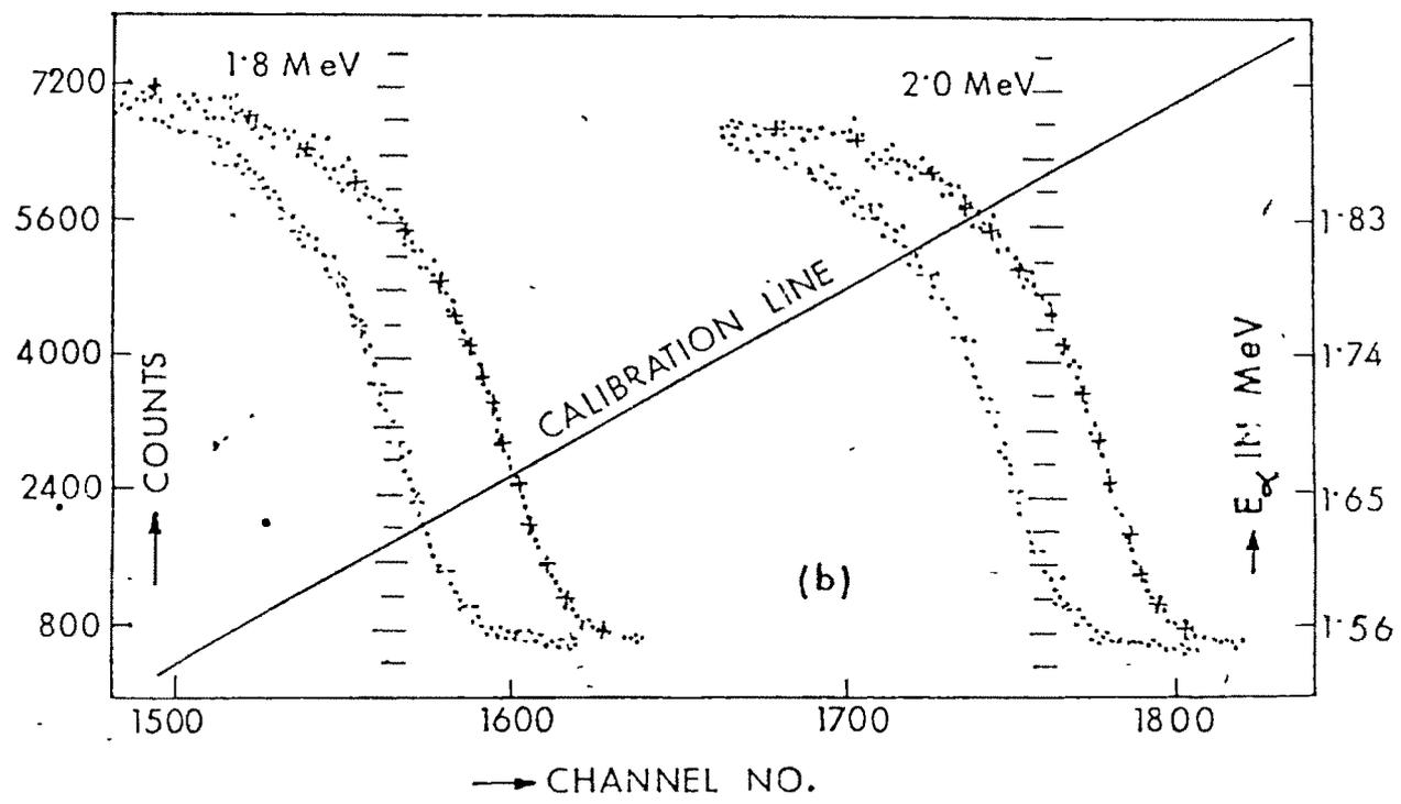
Fig. (2.1) : (a) A schematic sketch of the scattering of  $\alpha$ -particles for target thickness measurement, (b) detector spectrum for blank Ta (dots with crosses) and Ta covered with target film (dots alone). The scale on the right side is for detector calibration.
