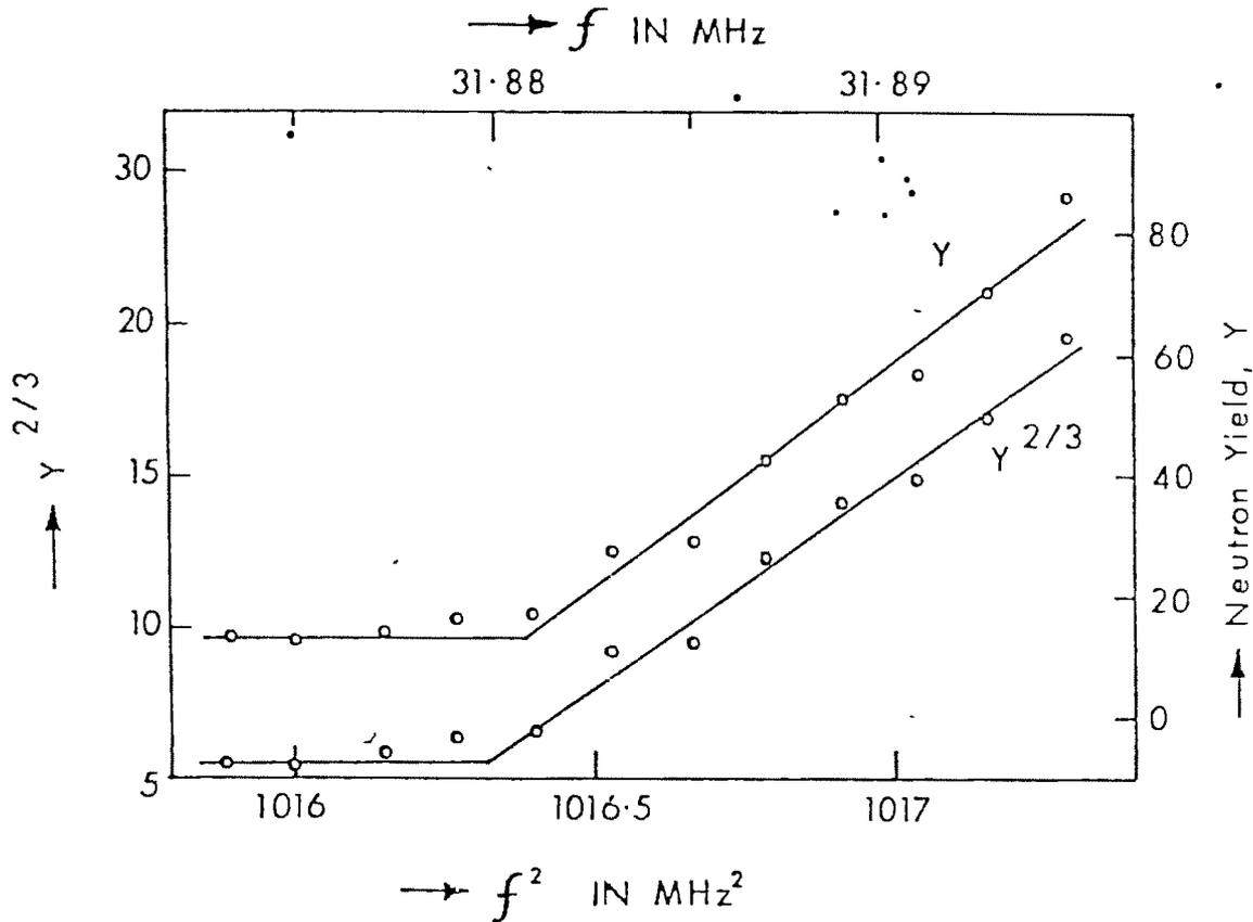
Fig. (2.3) Yield curve for the reaction  ${}^7\text{Li} (p,n) {}^7\text{Be}$  as a function of NMR frequency to determine the accelerator calibration constant.
