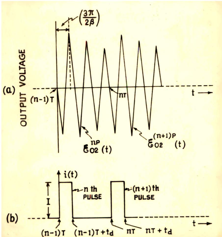
Fig.4.1 Schematic diagram of the multiplier output (a) excited by the  $n$ th and  $(n + 1)$ th current pulses (b).
