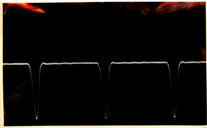
Fig.7.3 Oscillogram of the plate current pulse waveform at the anode of EL80F multiplier. Time scale is 0.2 \mu \text{ sec/cm} .
