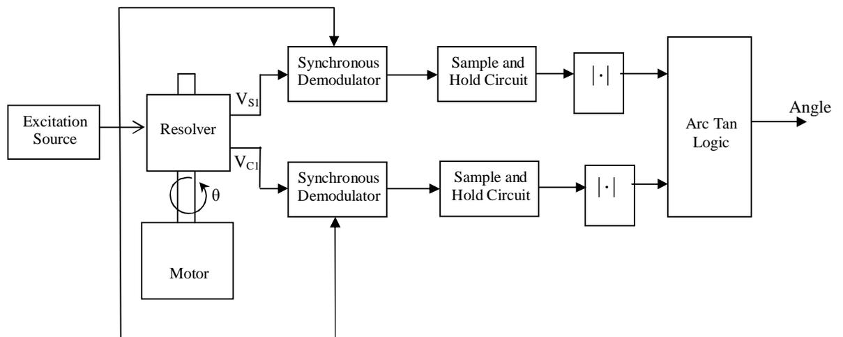
Figure 3.2 Arctangent algorithm based RDC
