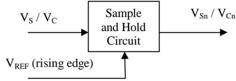
Figure 3.4 Sample and hold circuit
