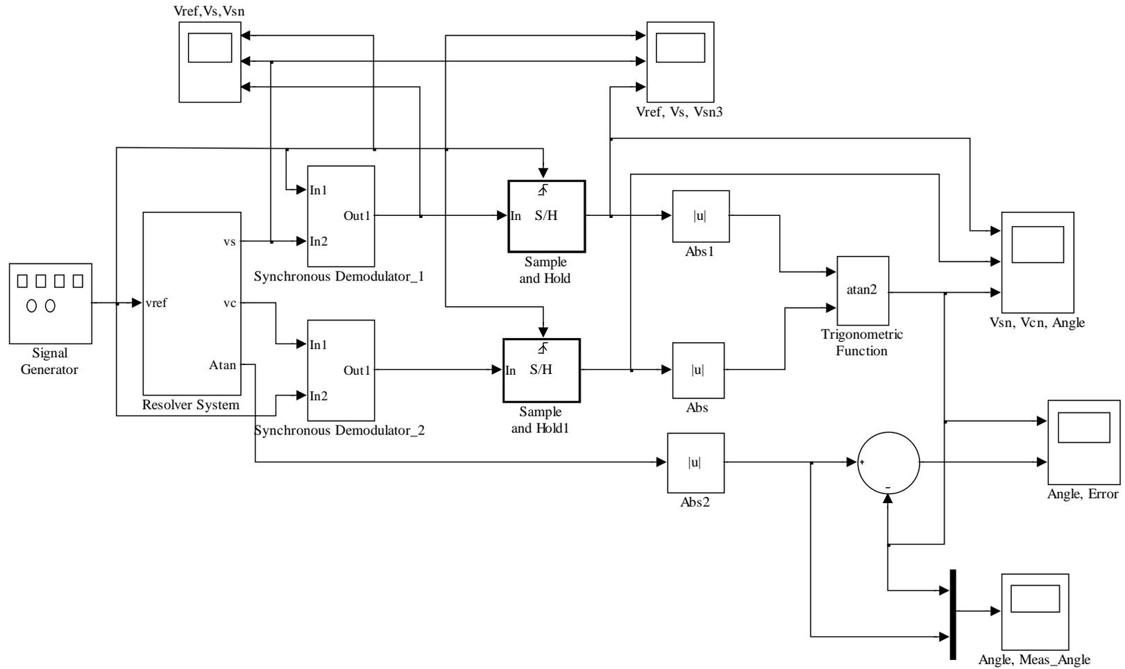
Figure 3.5 MATLAB<sup>®</sup> SIMULINK<sup>®</sup> model of RDC using Arctangent algorithm
