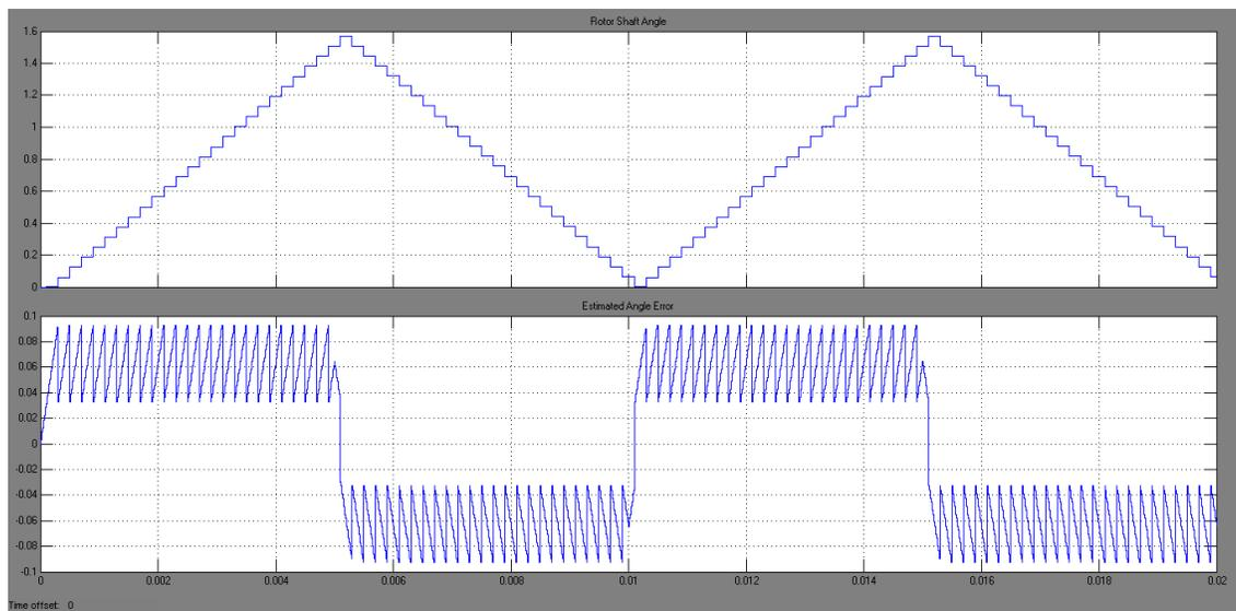
Figure 3.21 Measured rotor angle and rotor angle error
