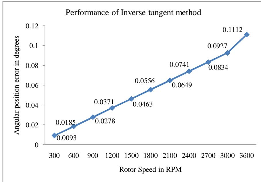
Figure 3.22 Graph between rotor angular position error and rotor speed
