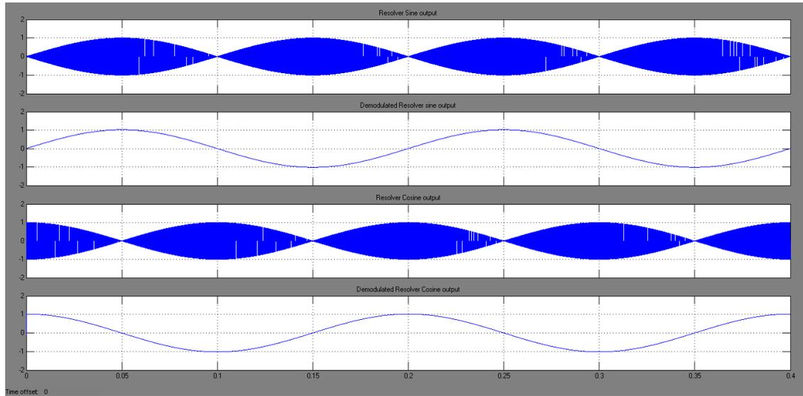
Figure 3.8 SIN output, demodulated SIN, COS output and demodulated COS signals
