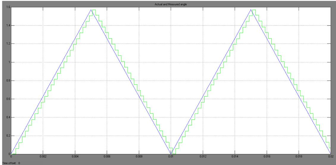
Figure 3.20 Actual rotor angle (blue) and measured rotor angle (green)
