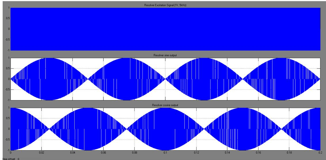
Figure 3.12 Square wave excitation signal, SIN and COS outputs of the resolver
