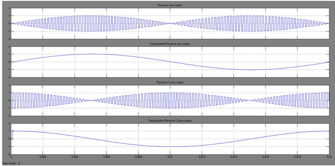
Figure 3.18 SIN output, demodulated SIN, COS output and demodulated COS signals
