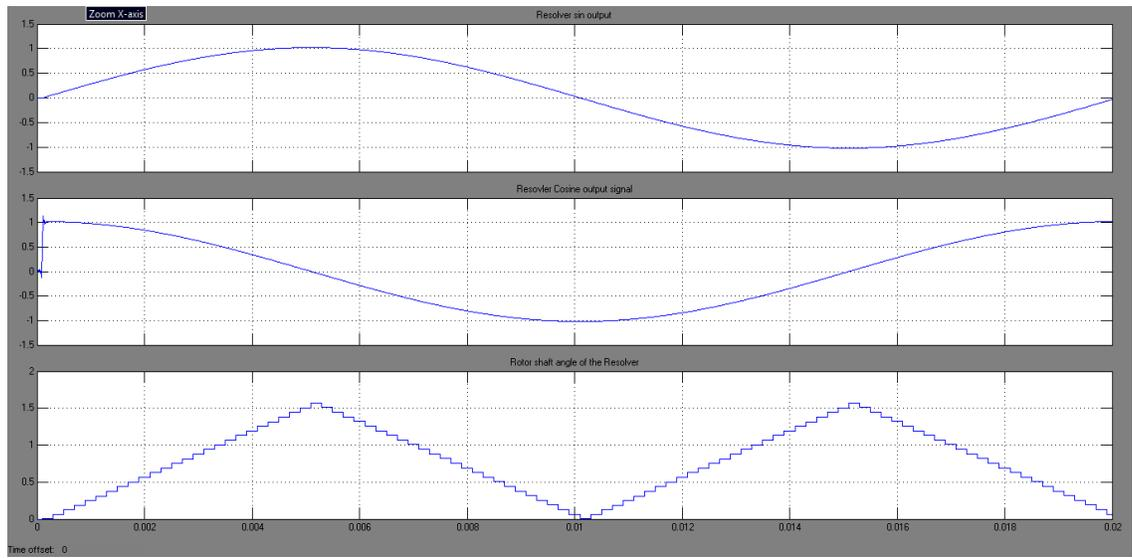
Figure 3.19 Sampled SIN and COS outputs and measured rotor shaft angle
