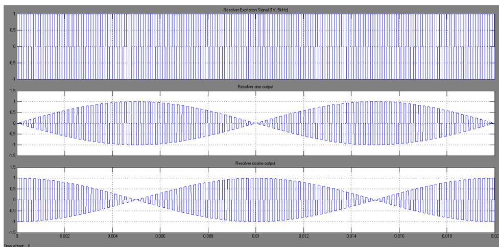
Figure 3.17 Square wave excitation signal, SIN and COS outputs of the resolver
