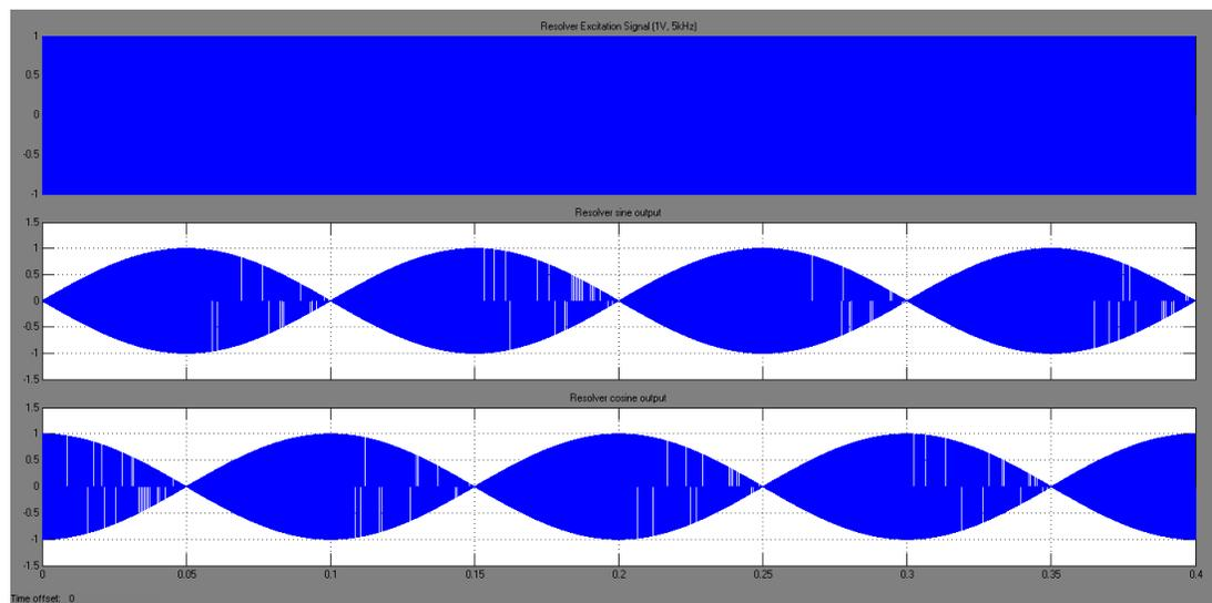
Figure 3.7 Square wave excitation signal, SIN and COS outputs of the resolver
