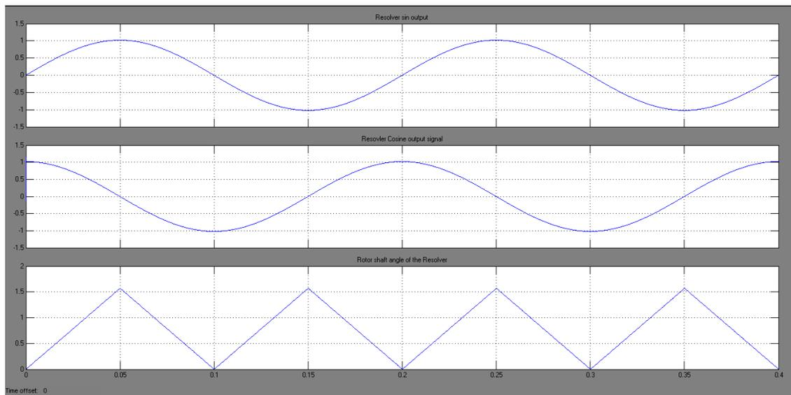
Figure 3.9 Sampled SIN and COS outputs and measured rotor shaft angle
