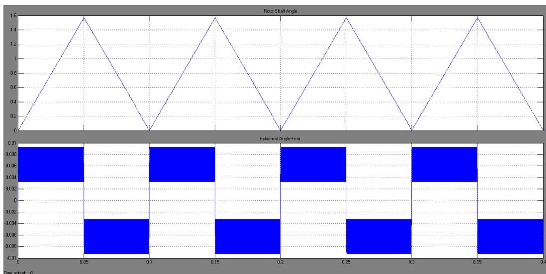
Figure 3.11 Measured rotor angle and rotor angle error
