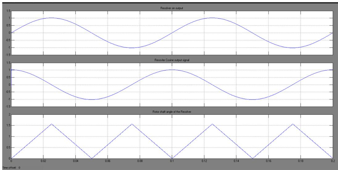
Figure 3.14 Sampled SIN and COS outputs and measured rotor shaft angle
