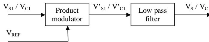
Figure 3.3 Synchronous demodulator
