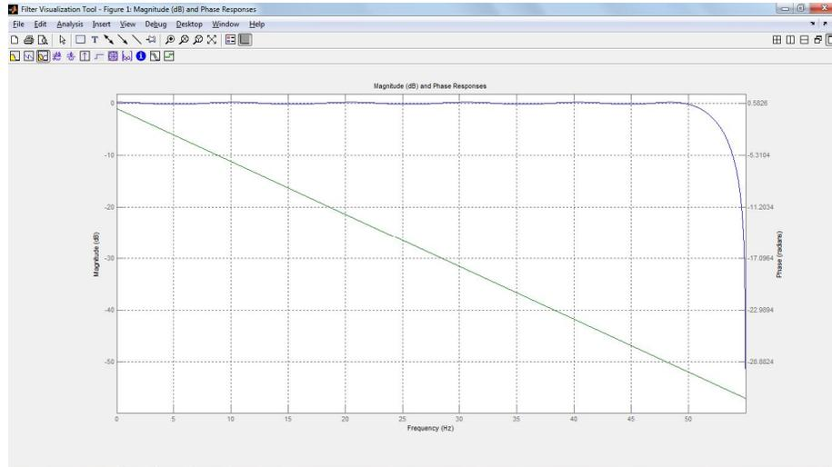
Figure 3.6 Frequency response of low pass filter
