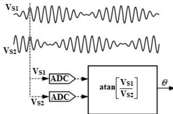
Figure 3.1 Angle extraction using Arctangent algorithm
