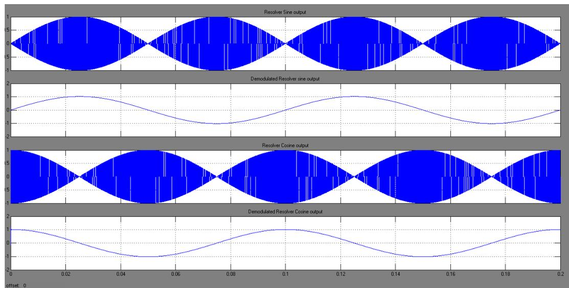
Figure 3.13 SIN output, demodulated SIN, COS output and demodulated COS signals
