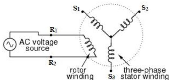
Figure 1.1 Modern schematic diagram of a synchro
