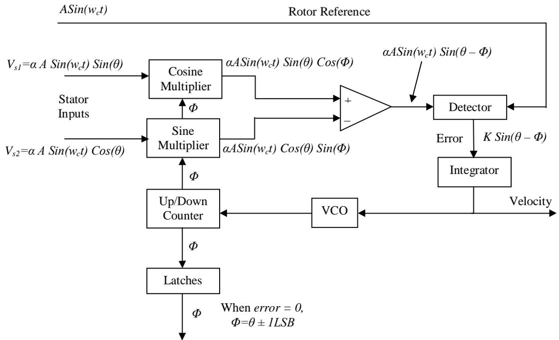
Figure 1.14 Resolver to digital converter based on ATO Technique
