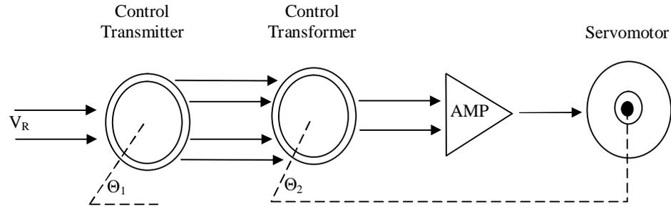
Figure 1.6 Electromechanical Servo mechanism
