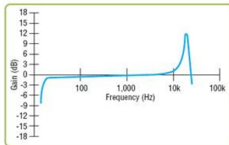
Figure 1.3 Frequency response of a resolver
