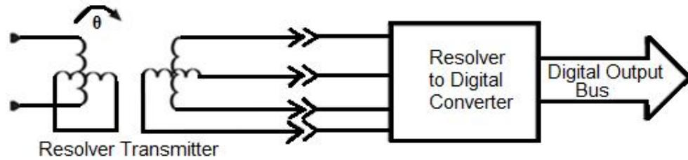
Figure 1.12 Digital data transmission of a resolver system
