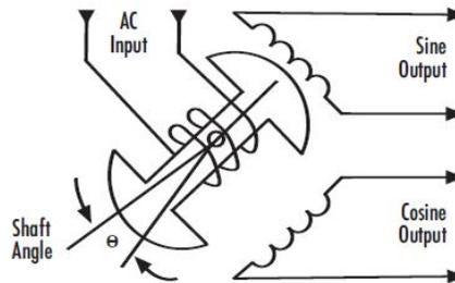
Figure 1.8 Schematic of a Resolver
