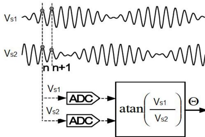
Figure 1.13 Angle extraction using Arctangent Method
