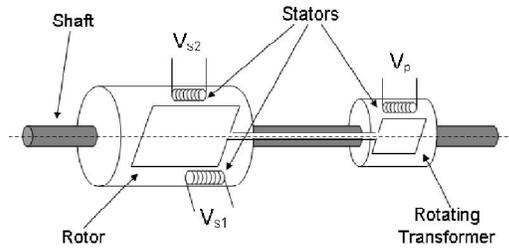
Figure 1.9 Internal view of a resolver
