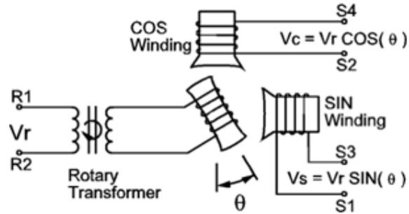
Figure 1.4(b) Schematic diagram of brushless resolver control transmitter
