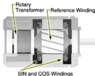
Figure 1.4(a) Cross section of brushless resolver
