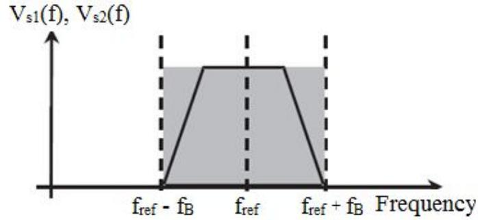
Figure 1.11 Amplitude spectrum of resolver signals  $V_{s1}$ ,  $V_{s2}$
