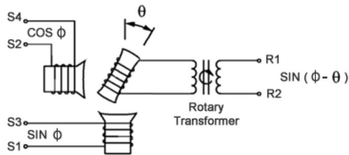
Figure 1.5 Schematic of brushless resolver control transformer
