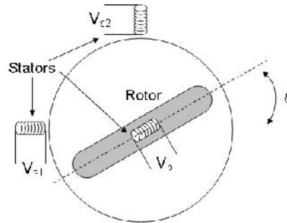
Figure 1.10(a) Equivalent cross sectional view
