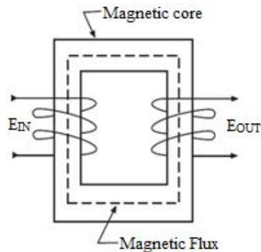
Figure 1.7 Schematic of a Stationary transformer
