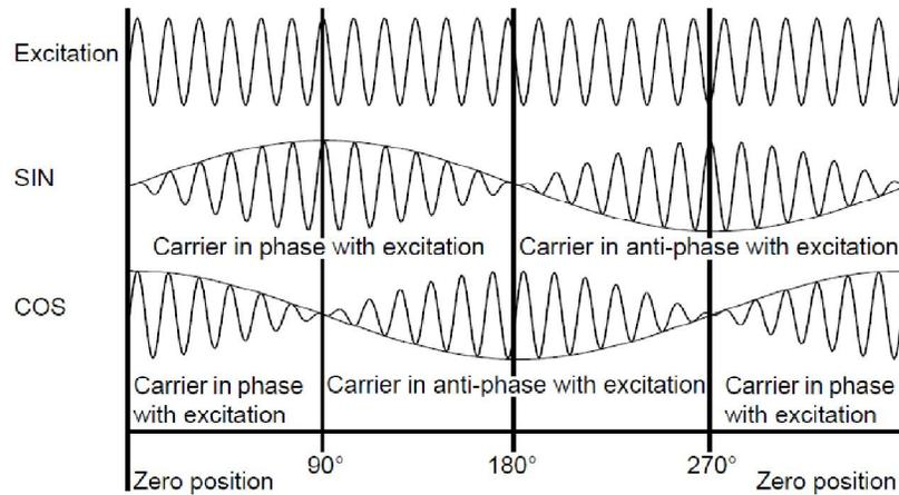
Figure 1.10(b) Resolver excitation and output signals
