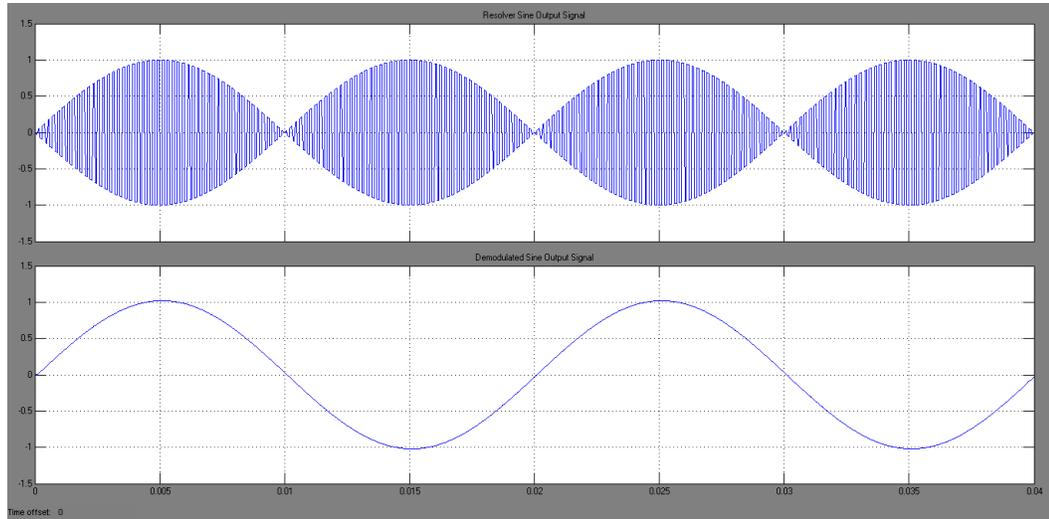
Figure 4.12 SIN output, demodulated SIN, COS output and demodulated COS signals
