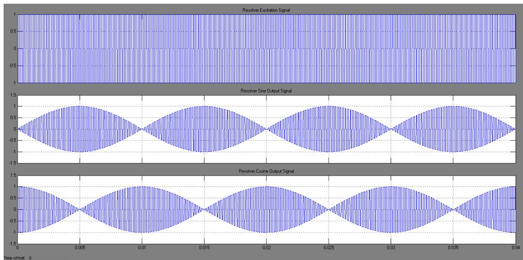
Figure 4.11 Square wave excitation signal, SIN and COS outputs of the resolver
