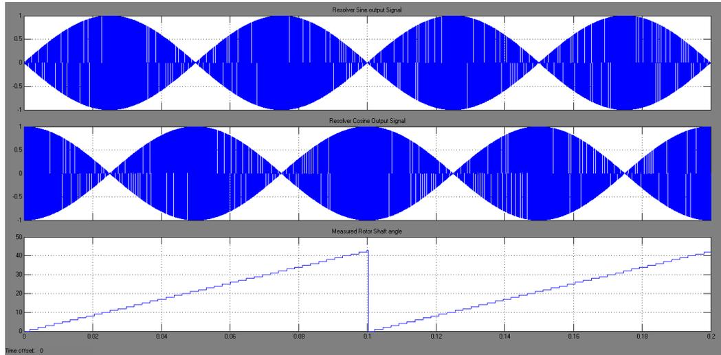
Figure 4.10 SIN, COS modulated signals of resolver and measured rotor shaft angle
