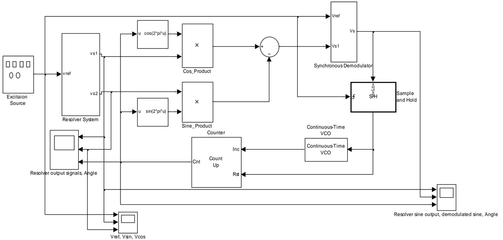
Figure 4.3 MATLAB® SIMULINK® model of RDC using ATO algorithm
