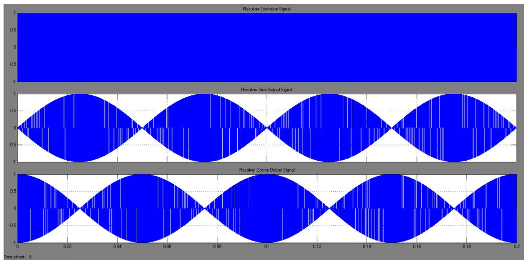
Figure 4.8 Square wave excitation signal, SIN and COS outputs of the resolver
