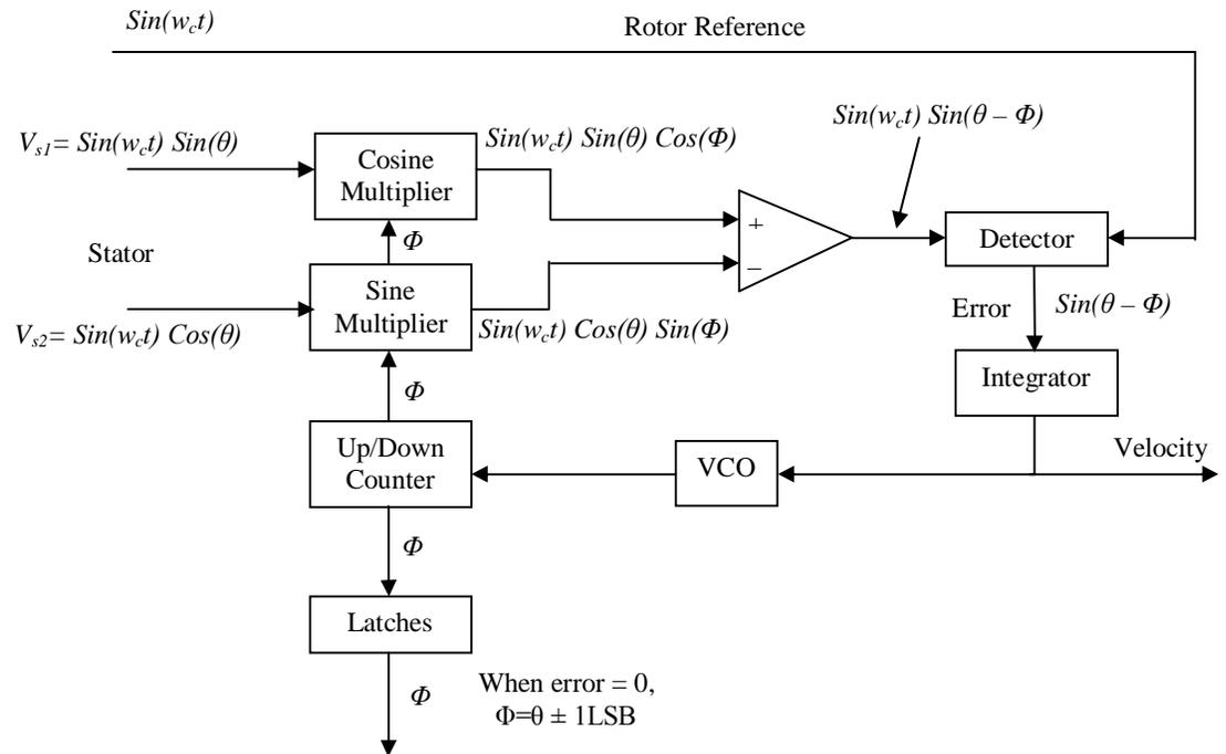
Figure 4.2 Structure of ATO based Resolver to Digital Converter
