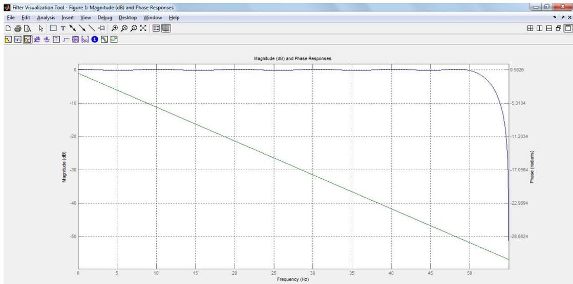
Figure 4.4 Magnitude and phase response of Low pass filter
