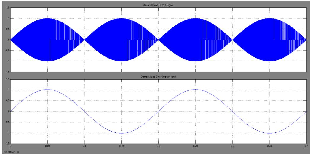
Figure 4.6 SIN output, demodulated SIN, COS output and demodulated COS signals
