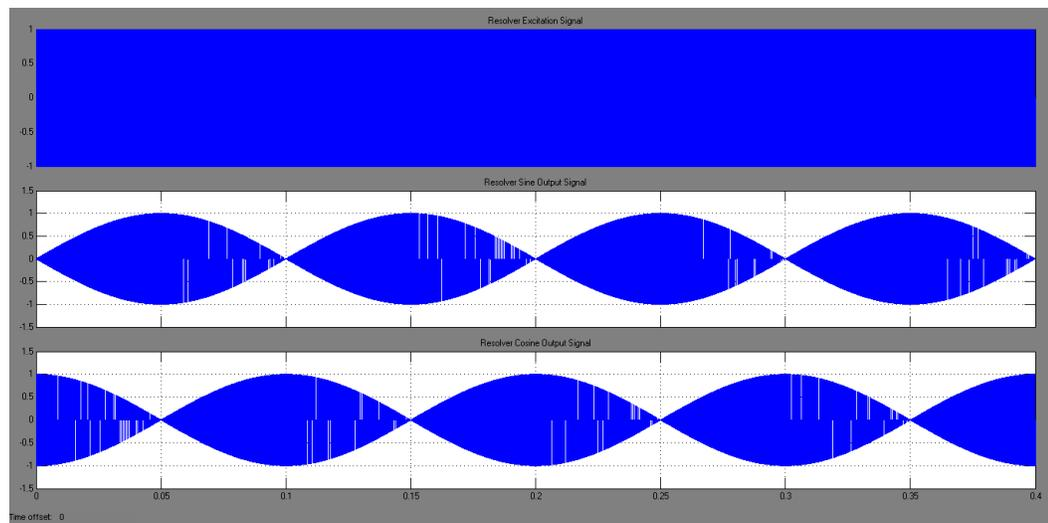
Figure 4.5 Square wave excitation signal, SIN and COS outputs of the resolver
