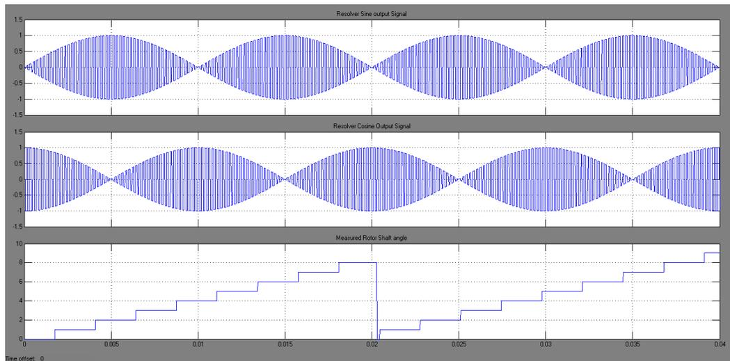
Fig: 3.23 Sine, Cosine modulated signals of resolver and measured rotor shaft angle
