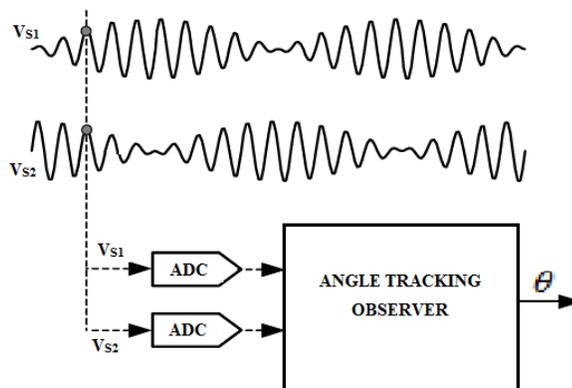
Figure 4.1 Angle extraction using angle tracking observer
