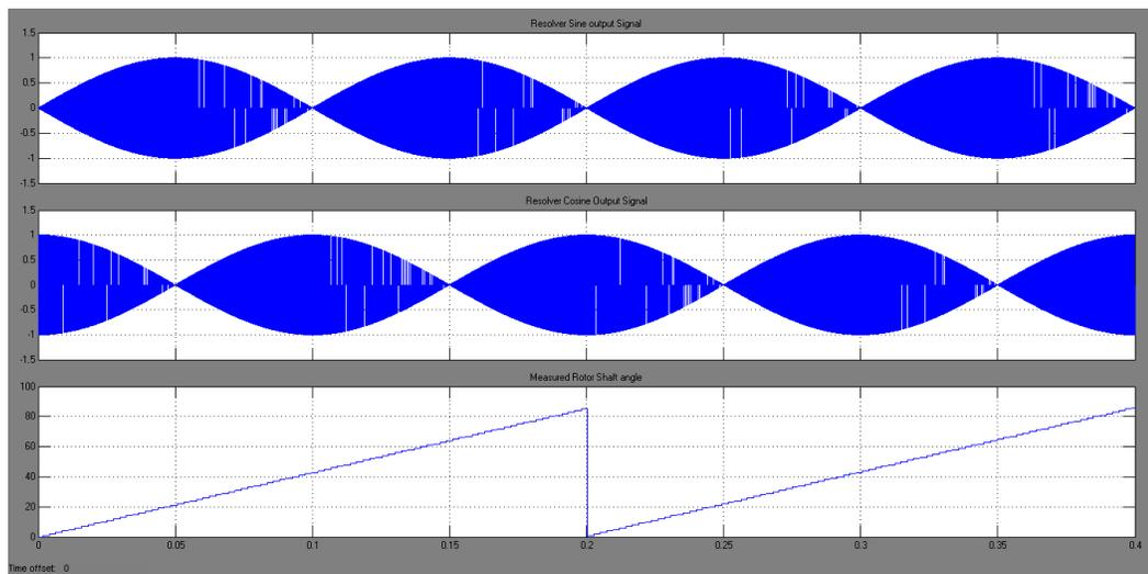
Figure 4.7 SIN, COS modulated signals of resolver and measured rotor shaft angle
