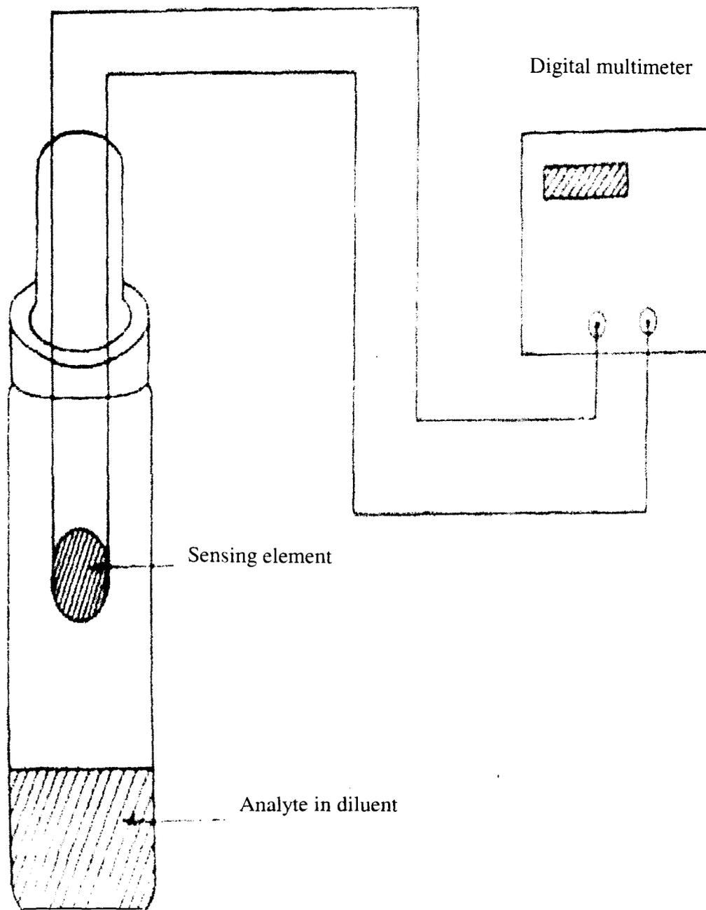
**Fig. 2.2** Schematic representation of sensing measurement.
