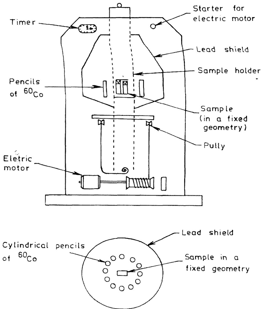
**Fig. 2.1** Cross section and top view of the gamma source.
