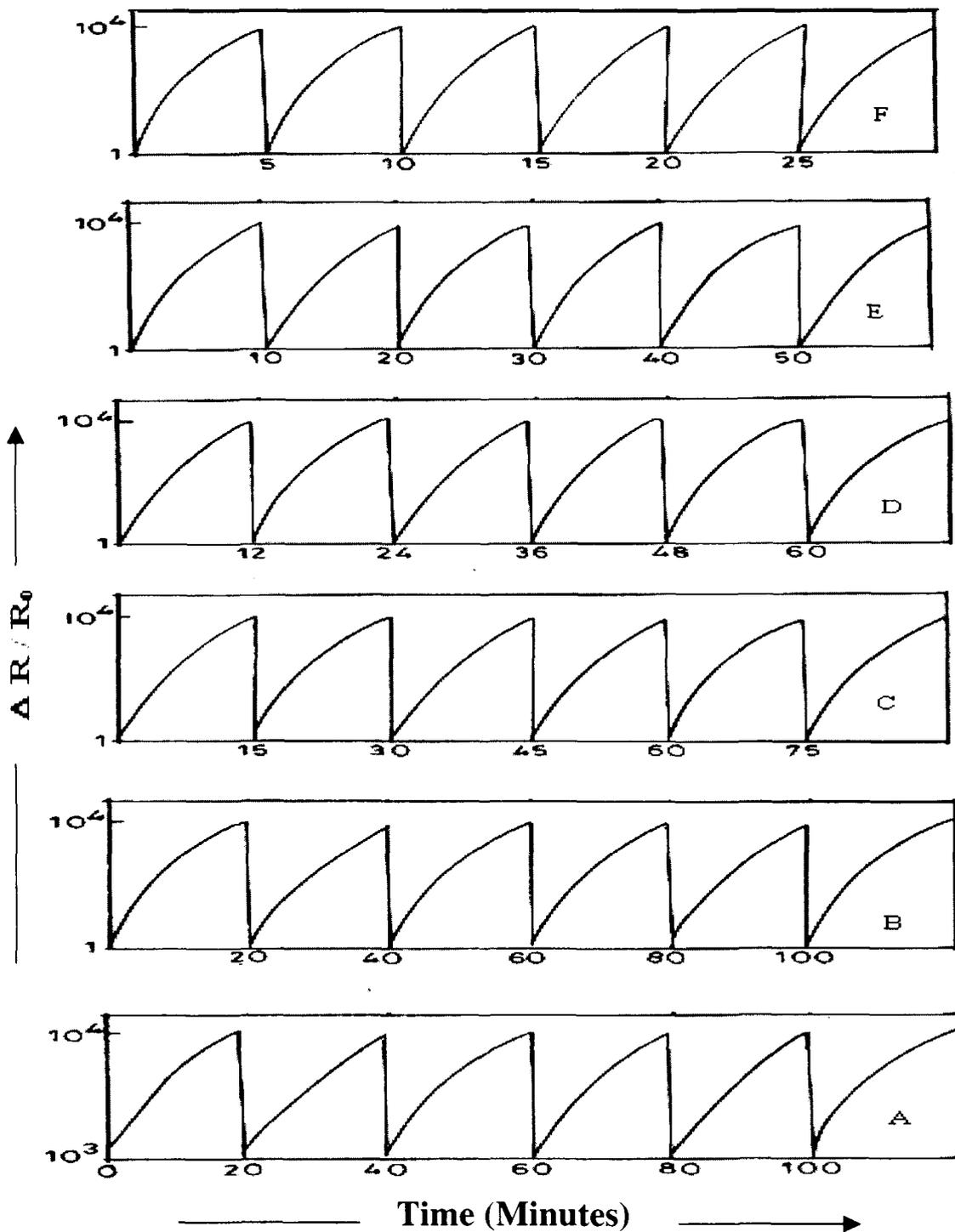
**Fig. 4.8** Blank Pani exposed to A) 600 ppm and Au-Pani nanocomposite exposed to B) 1, C) 5, D) 10, E) 100 and F) 600 ppm concentrations of methanol.
