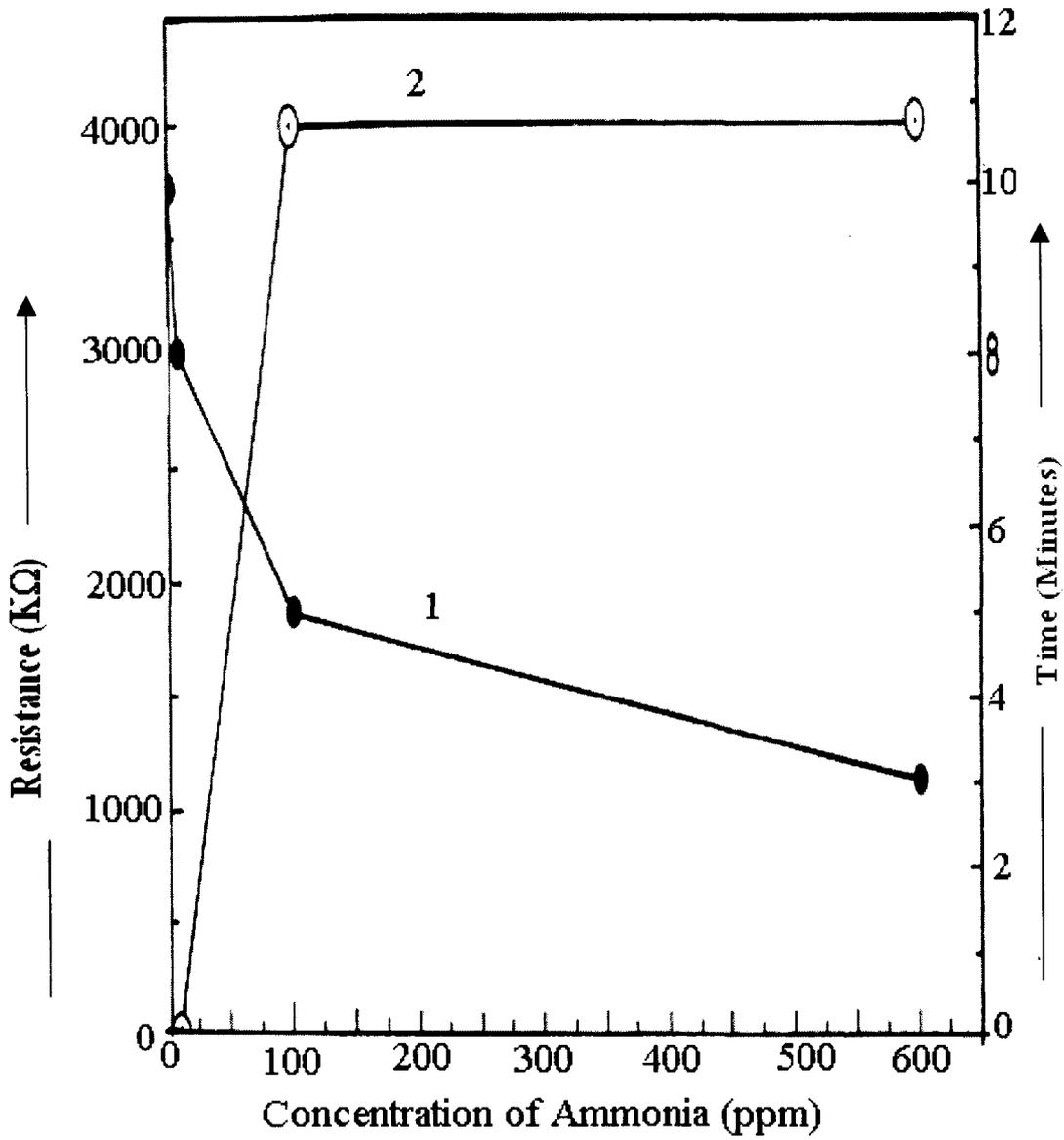
**Fig. 4.6** A plot of concentration of ammonia vs 1) response time and 2) resistance.
