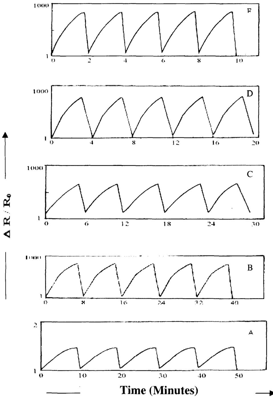
**Fig. 4.1** Pd-Pani nanocomposite exposed to various concentrations of methanol such as A) 50 ppm, B) 100 ppm and C) 2000 ppm.
