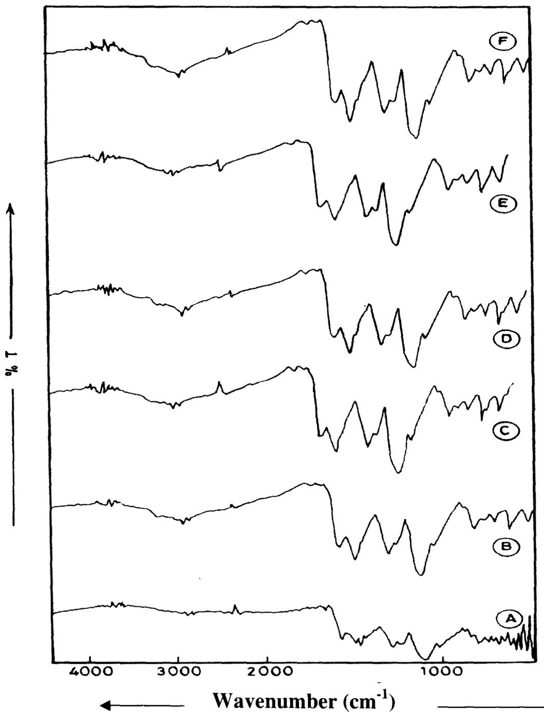
**Fig. 4.10** FT-IR spectra of A) unexposed Au-Pani nanocomposite along with the nanocomposite exposed to concentration of B) 1, C) 5, D) 10, E) 100 and F) 600 ppm methanol.
