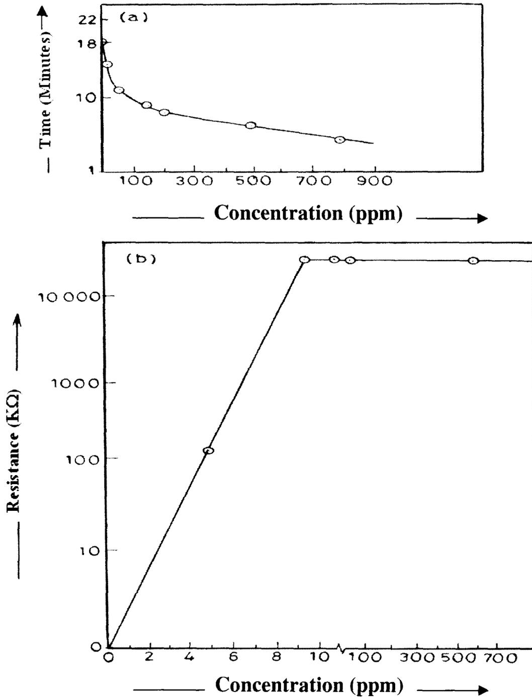
**Fig. 4.9** A plot of concentration of methanol vapour against a) response time and b) resistance of Au-PANI nanocomposite.
