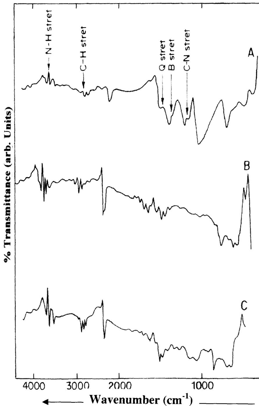
**Fig. 4.3** FT-IR spectra of A) unexposed Pd-Pani nanocomposite and those exposed to various concentrations of methanol vapours such as B) 1 and C) 2000 ppm.
