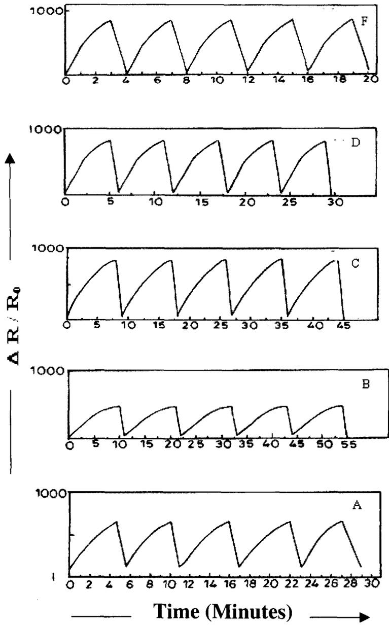
**Fig. 4.5** Blank Pani exposed to A) 600 ppm and Ag-Pani nanocomposite exposed to B) 1, C) 10, D) 100 and E) 600 ppm concentrations of ammonia.
