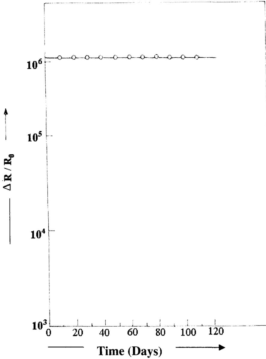
**Fig. 4.4** A plot showing long term stability of Pd-Pani nanocomposite as methanol vapour sensor.
