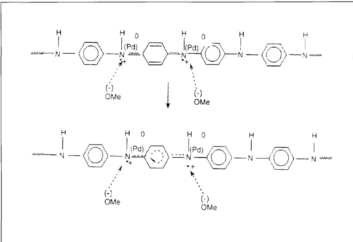
Scheme 1. Schematic representation of sensing mechanism.
