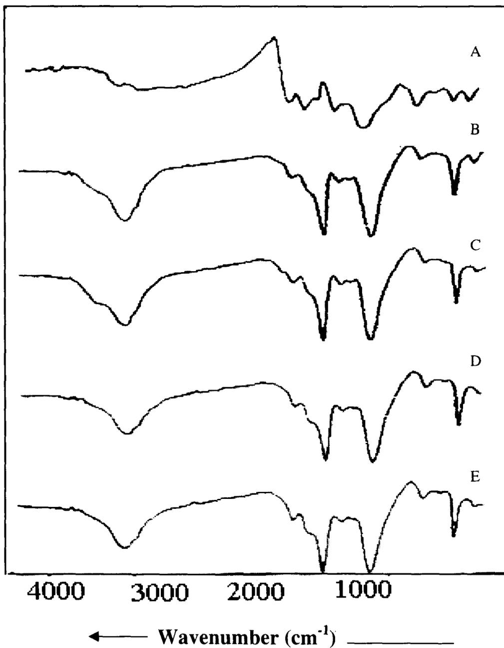
**Fig. 4.7** Blank Pani exposed to A) 600 ppm and Ag-Pani nanocomposite exposed to B)1, C) 10, D) 100 and E) 600 ppm concentrations of ammonia.
