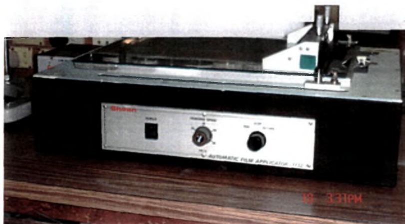
Figure 5.1 Sheen automatic film applicator.
