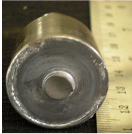
Tool pin failure at 1400 rpm
