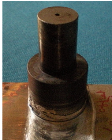
Tool struck at rotational speed of 1100 rpm and welding speed of 100 mm/min
