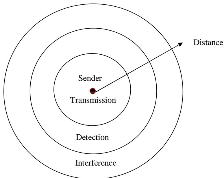
**Figure 1.1 Signal propagation range**
