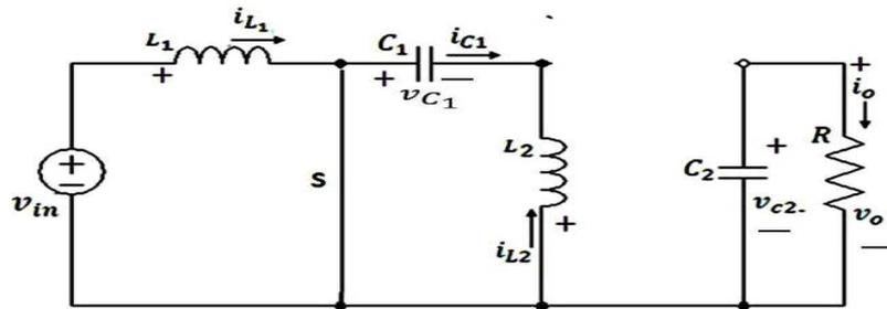
**Figure 1.2 SEPIC converter during switch in ON condition**
