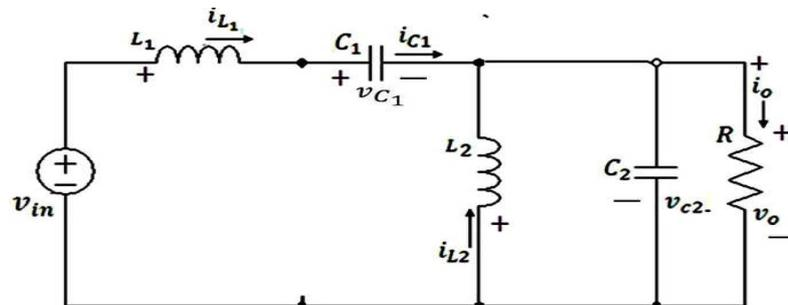
**Figure.1.3 SEPIC converter during switch in OFF condition**
