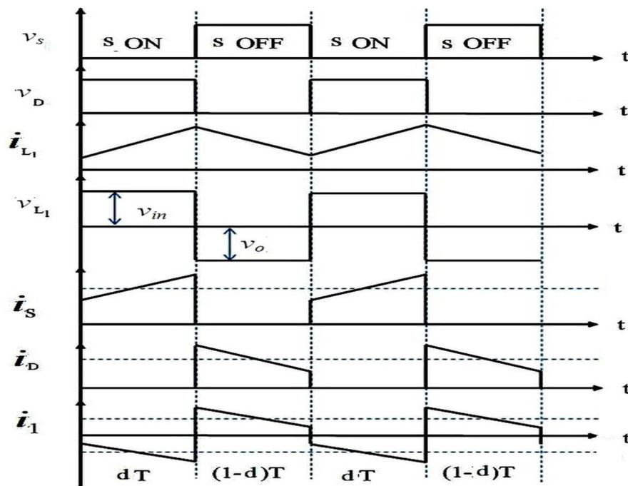
**Figure 1.3a Waveforms of different currents and voltages in SEPIC**
