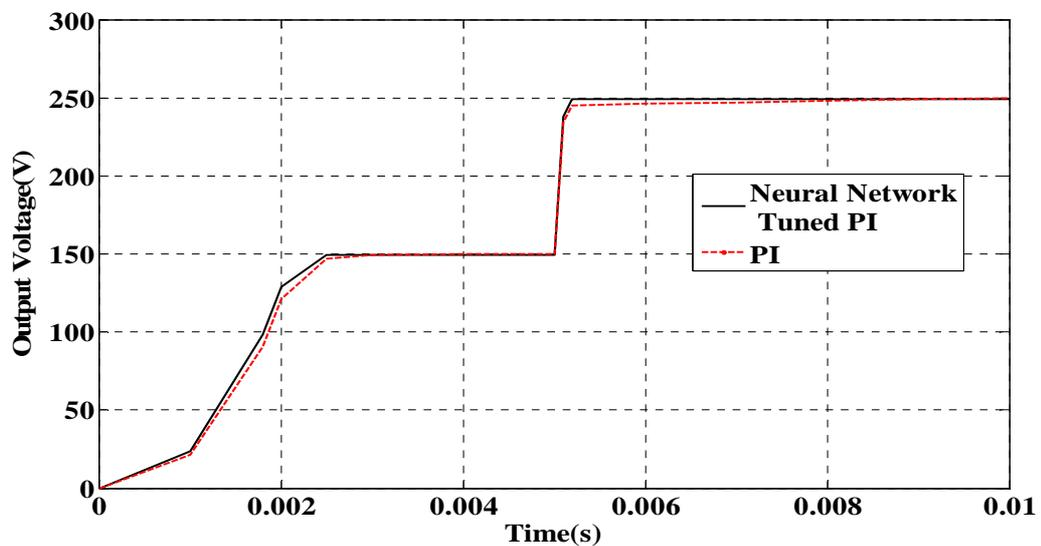
**Figure 3.8 Response while changing reference output voltage using NN tuned PI controller and PI controller**
