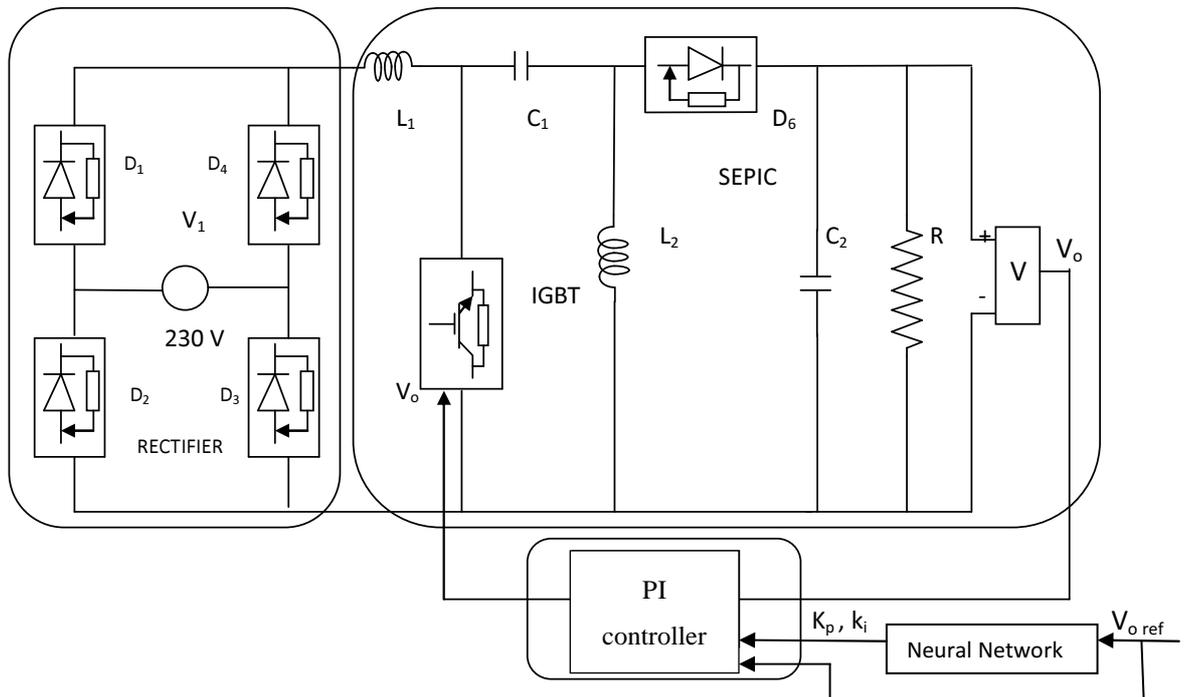
**Figure 3.6 Simulation circuit for SEPIC Converter with NN tuned PI controller**
