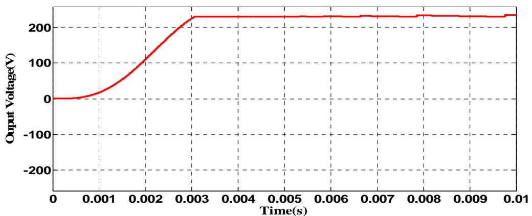
**Figure 3.7 SEPIC output voltage using NN tuned PI controller**
