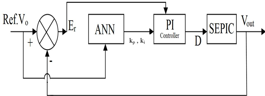
**Figure 3.2 Closed loop control of SEPIC**
