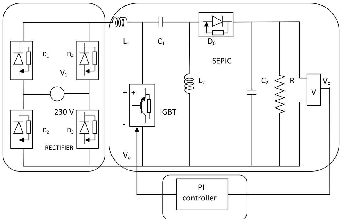
**Figure 3.3 Simulation Circuit for SEPIC converter with PI controller**
