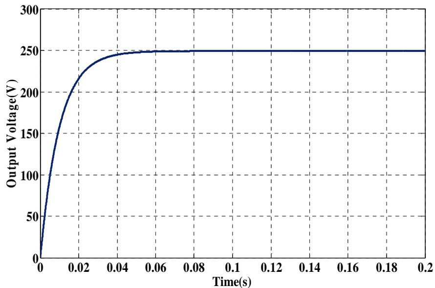
**Figure 3.5 SEPIC output voltage using PI controller**
