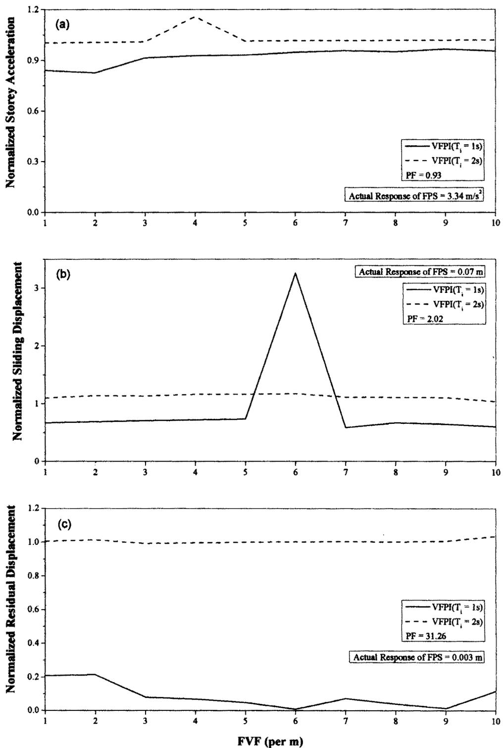
**Figure 4.5: Responses normalized with that of FPS ( $T_b = 2$  s) for MDOF system subjected to El Centro 1940 (N-S) earthquake, ( $\mu = 0.05$ )**
