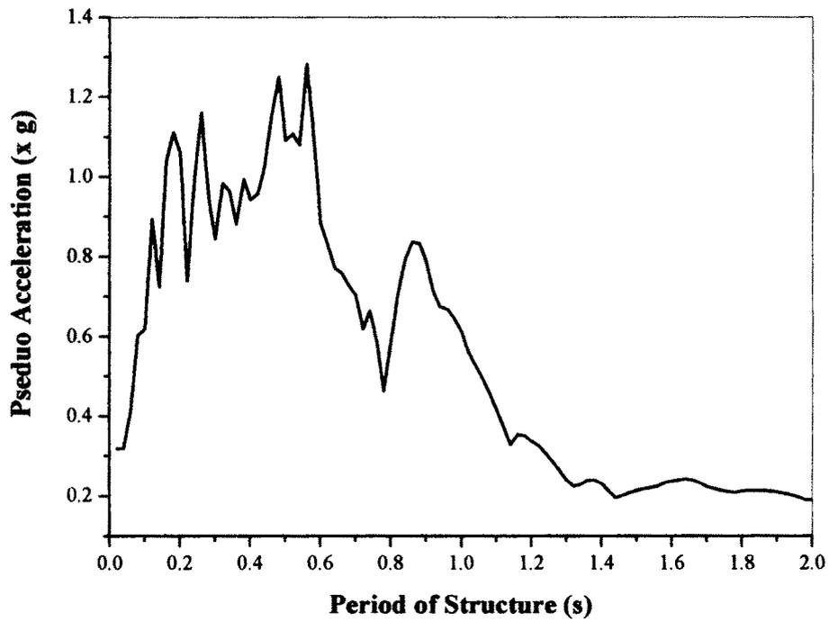
**Figure 4.2: Response spectra for El Centro 1940, N-S component ground motion**
