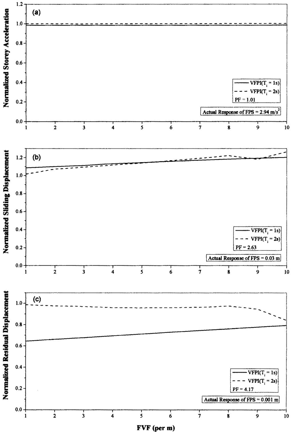
**Figure 4.4: Responses normalized with that of FPS ( $T_b = 2$  s) for SDOF system subjected to El Centro 1940 (N-S) earthquake, ( $\mu = 0.1$ )**
