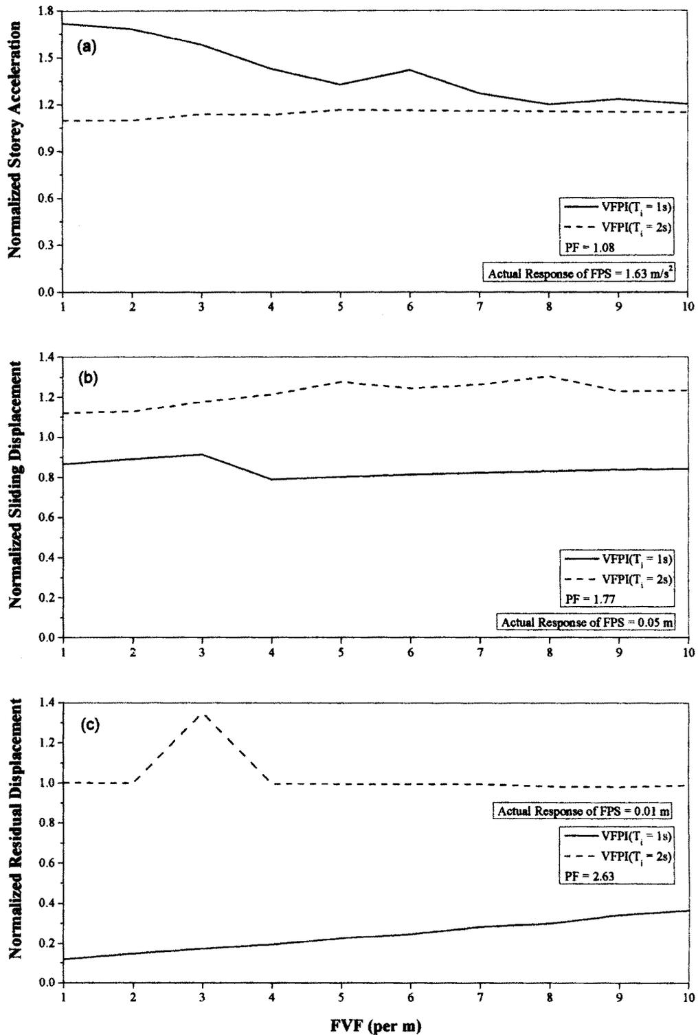
**Figure 4.3: Responses normalized with that of FPS ( $T_b = 2 \text{ s}$ ) for SDOF system subjected to El Centro 1940 (N-S) earthquake, ( $\mu = 0.05$ )**
