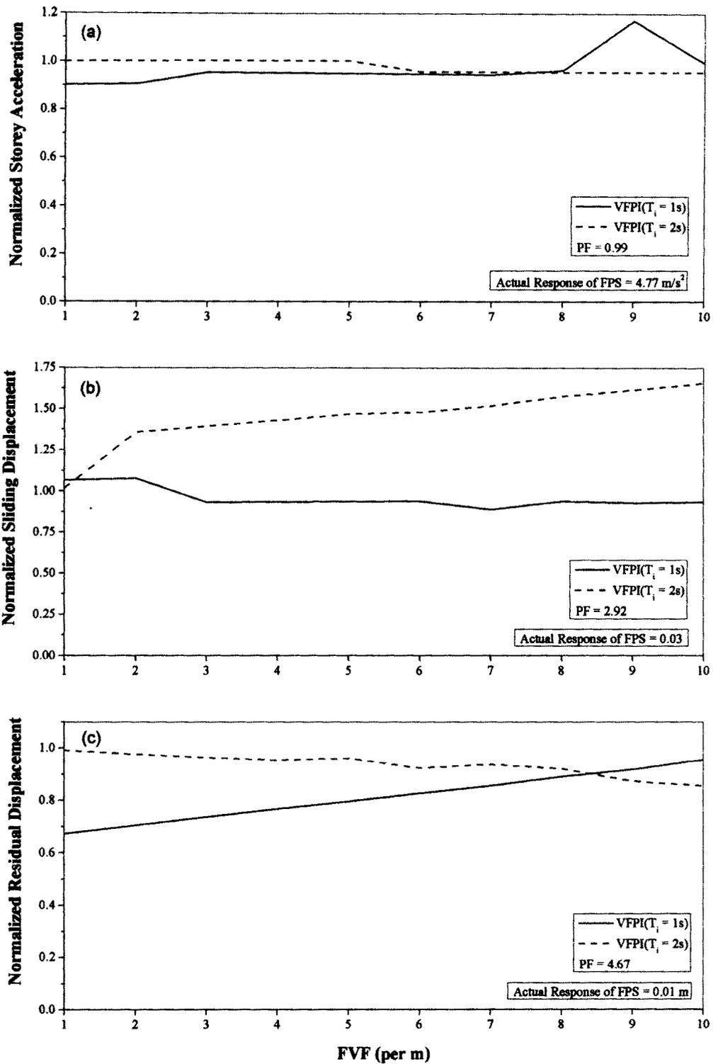
**Figure 4.6: Responses normalized with that of FPS ( $T_b = 2 \text{ s}$ ) for MDOF system subjected to El Centro 1940 (N-S) earthquake, ( $\mu = 0.1$ )**
