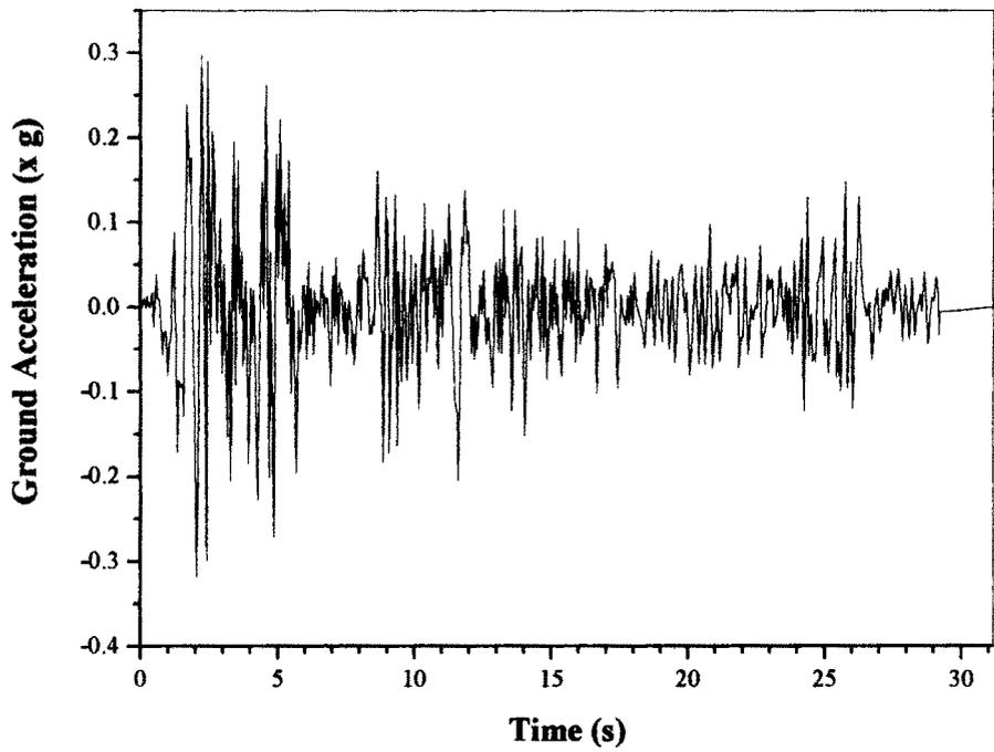
**Figure 4.1: Time history of El Centro 1940, N-S component ground motion**
