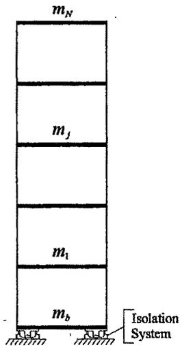
Figure 3.1: Lumped mass model with isolator
