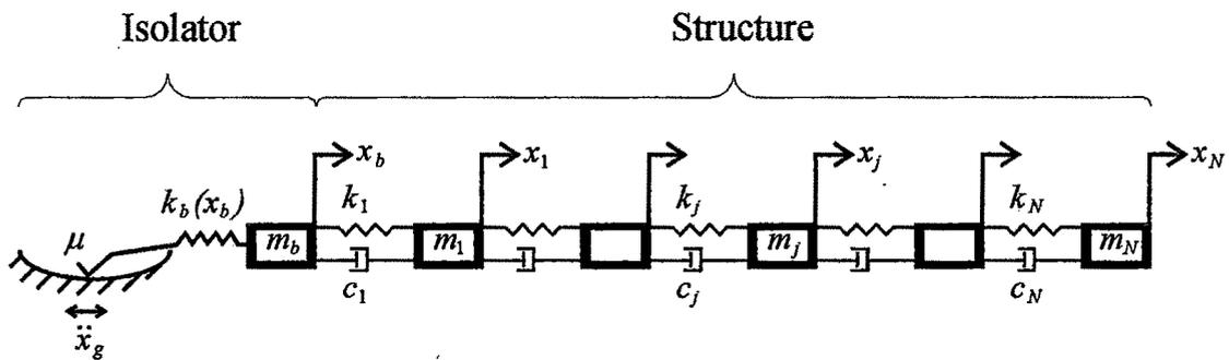
Figure 3.3: Analytical model of multi storied structure with base isolator
