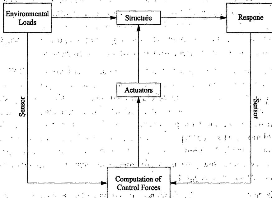
**Figure 1.2: Feedback control scheme of active control system**
