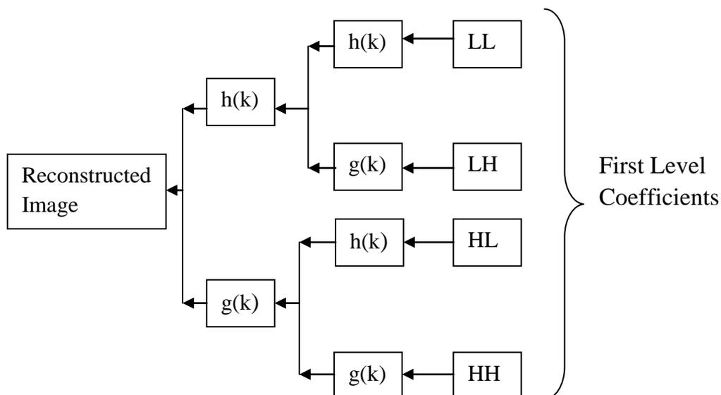
**Figure 1.5 One level reconstruction of UDWT**
