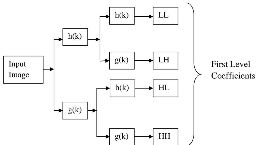
**Figure 1.4 One level decomposition of UDWT**
