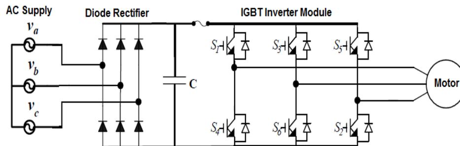
**Figure 1.2 Schematic of 3 $\phi$  IGBT inverter module connected with motor**
