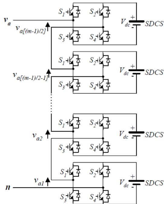
**Figure 1.4 Schematic diagram of single phase cascaded H-bridge multilevel inverter**
