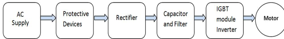
**Figure 1.1 Block diagram of adjustable AC drive system connected with an inverter**
