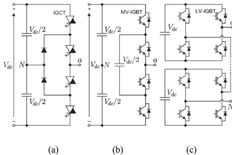
**Figure 1.3 Classic multilevel converter topologies (a) 3L-NPC featuring IGCTs (b) Three-level FC featuring MV-IGBTs (c) Five-level CHB featuring LV-IGBTs**
