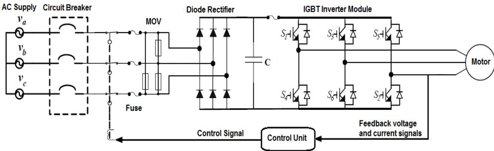
**Figure 1.5 Conventional fault diagnosis and protection system of voltage source inverter drive**
