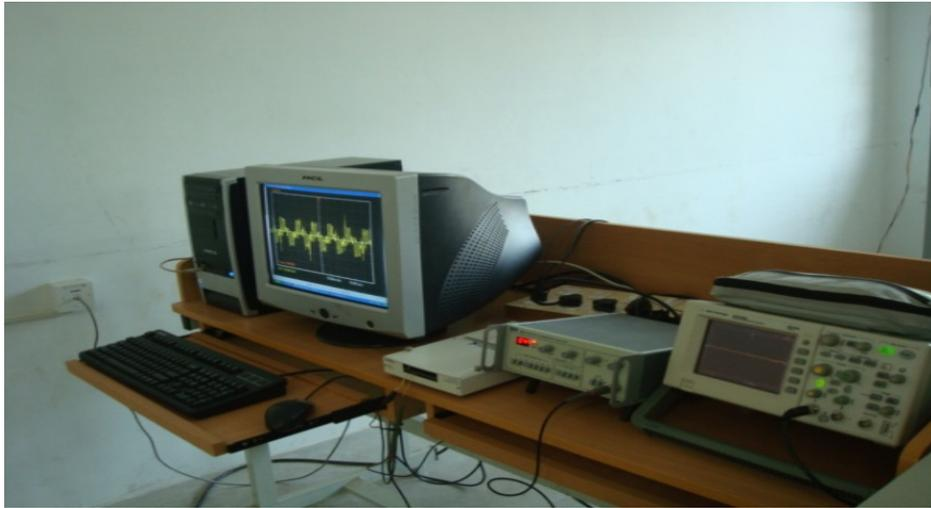
**Figure 5.7** Data acquisition system interfaced with LabVIEW software in PC
