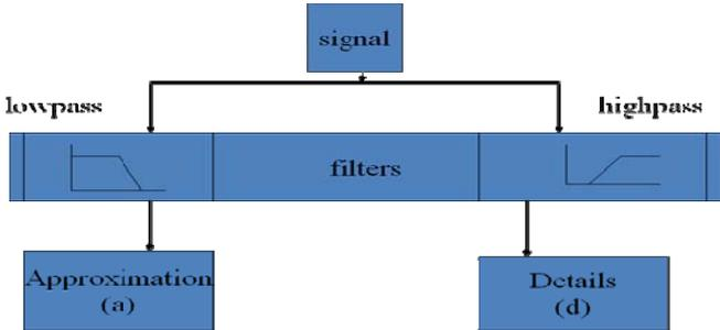
**Figure 3.4 Overview of signal decomposition using DWT**
