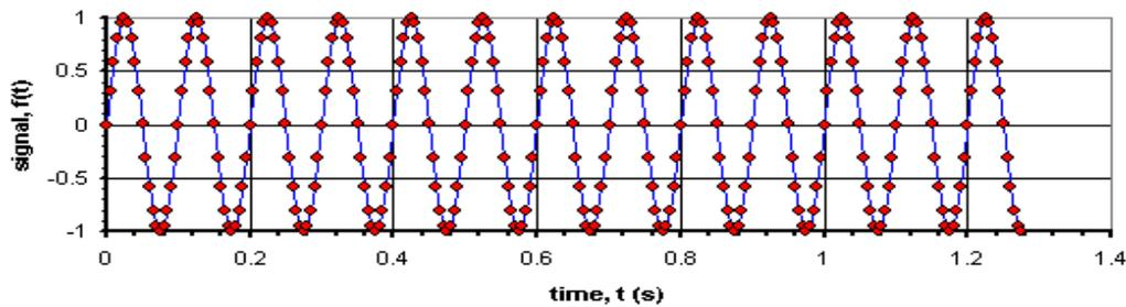
**Figure 3.1 Discretely sampled data of sine wave signal**
