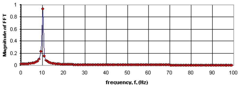
**Figure 3.2 Frequency spectrum of sine wave signal**
