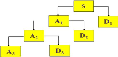
**Figure 3.5 Block diagram representation of wavelet coefficients**
