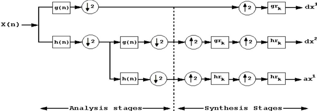
**Figure 3.3 Schematic implementation of MRSD**
