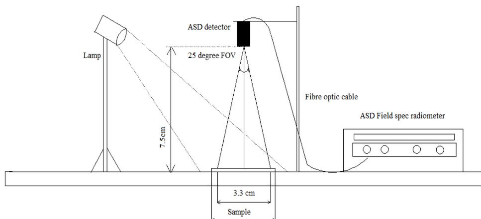
**Figure 3.8 Line sketch of the experimental setup for this study**
