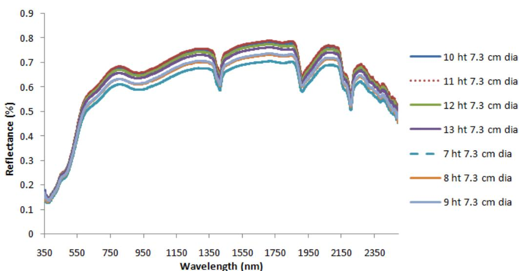
**Figure 3.5 Spectra of pure bentonite obtained from different heights of observation**
