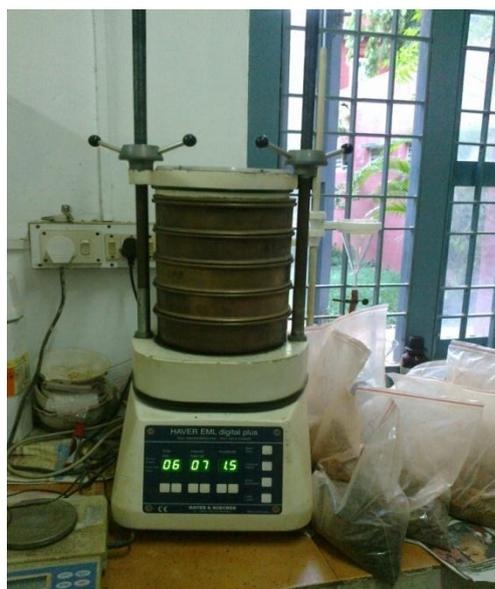
**Figure 3.9 Electronic sieve shaker and the instrument setup**
