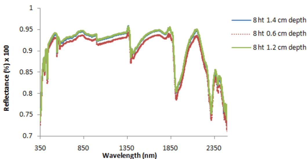
**Figure 3.7 Spectra of Kaolinite sample with different sample depth**
