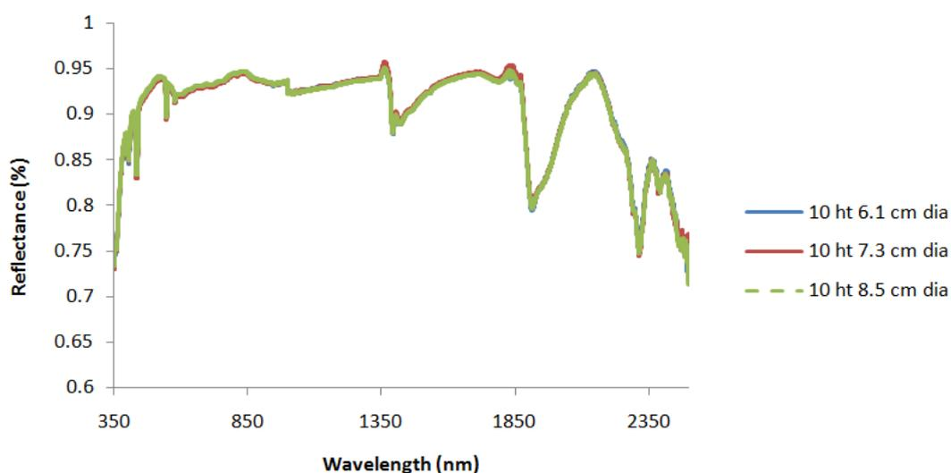
**Figure 3.6 Spectra of Kaolinite sample with different diameter of the sample spread**
