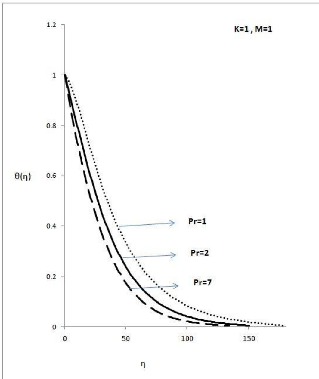
**Figure 4.3** Temperature profile for different values of Pr
