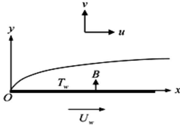
**Figure 4.1 Physical model and coordinate system**
