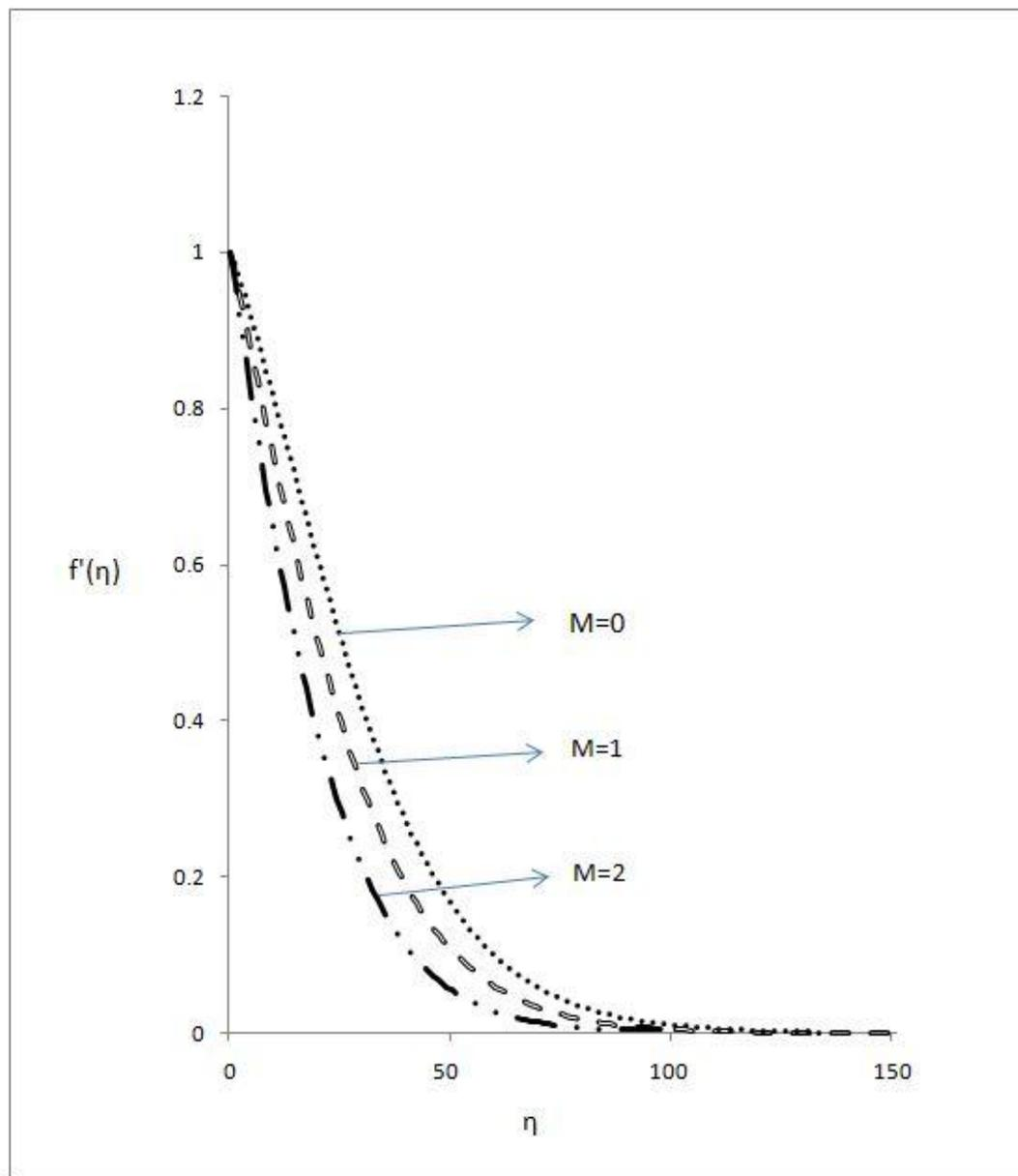
**Figure 4.2** Velocity profile for different values of  $M$
