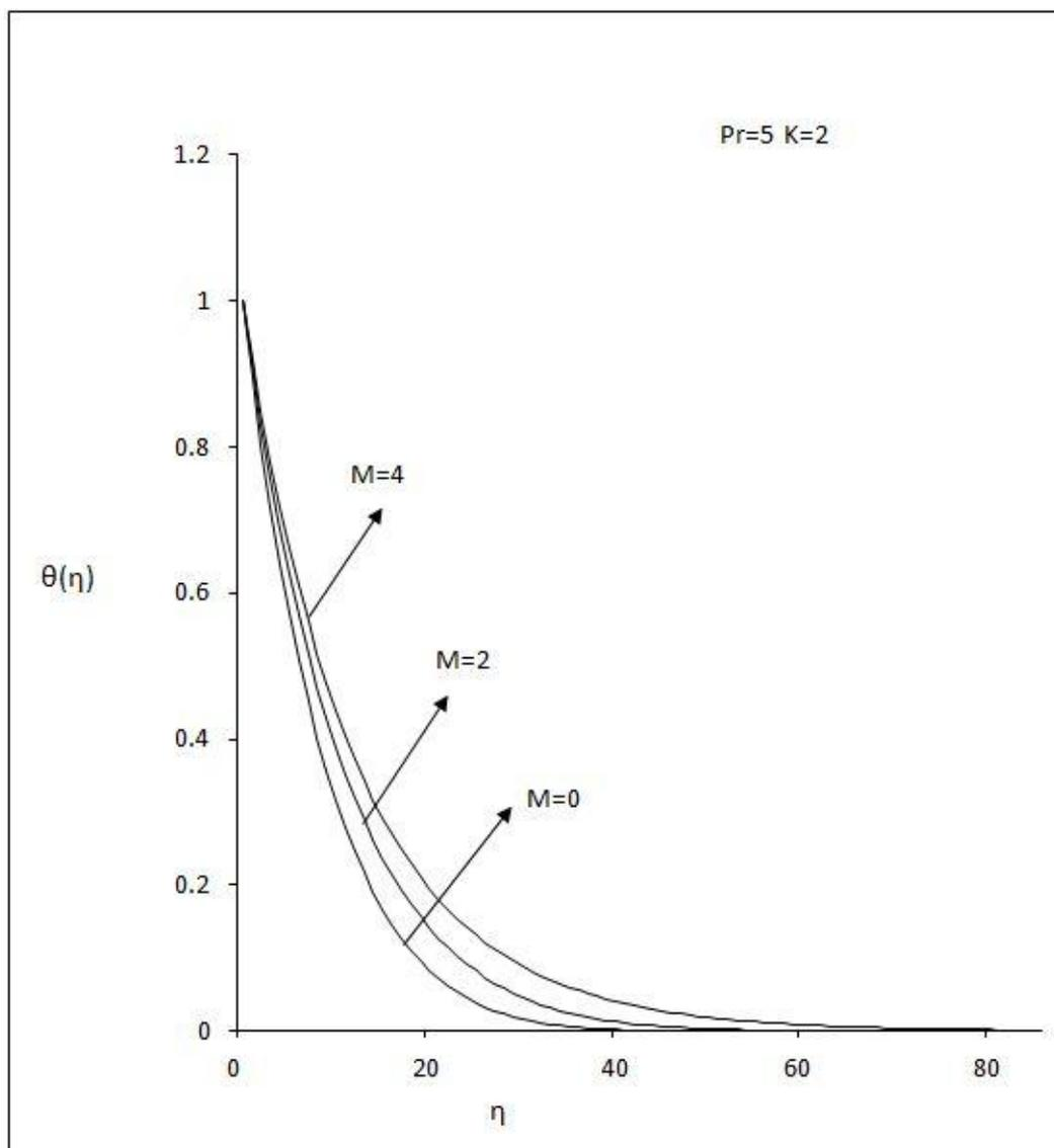
**Figure 4.5** Temperature profile for different values of  $M$
