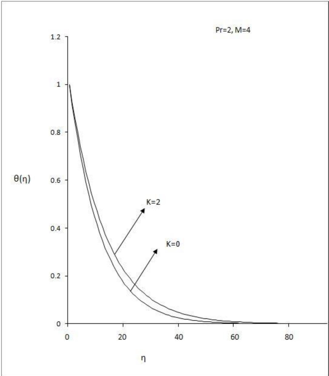
**Figure 4.4** Temperature profiles for different values of K
