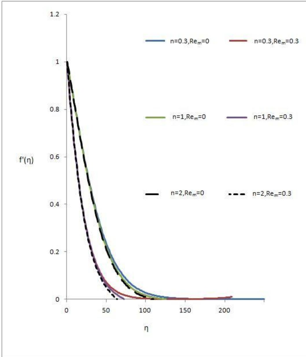
**Figure 2.3** Velocity profile against  $\eta$  for different values of  $n$  and  $Re_m$  with  $Pr = 0.02$ ,  $Ec = 0$  and  $\theta_r = 2.0$
