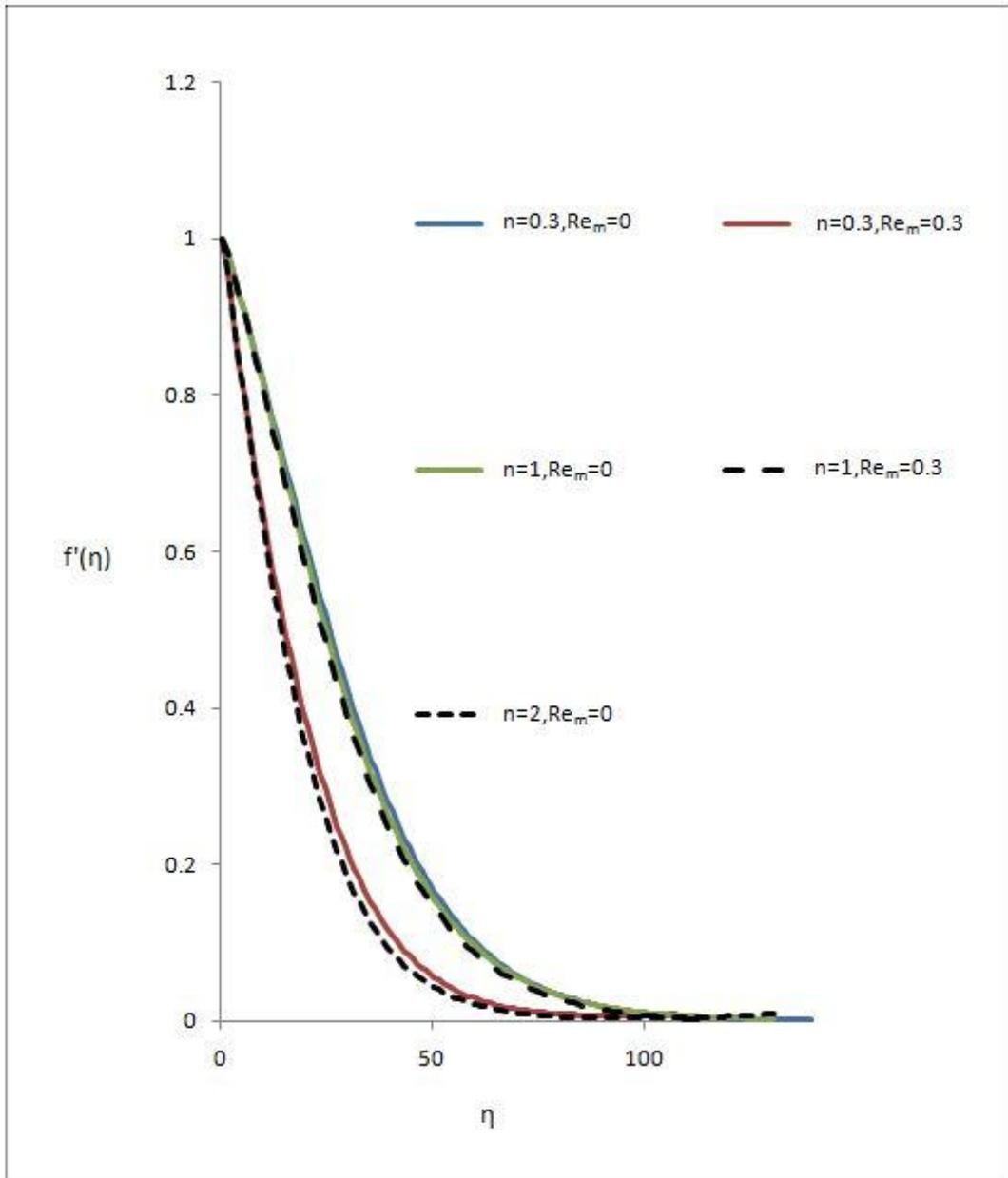
**Figure 2.2** Velocity profile against  $\eta$  for different values of  $n$  and  $Re_m$  with  $Pr=0.02$  and  $\theta_r = 2.0$
