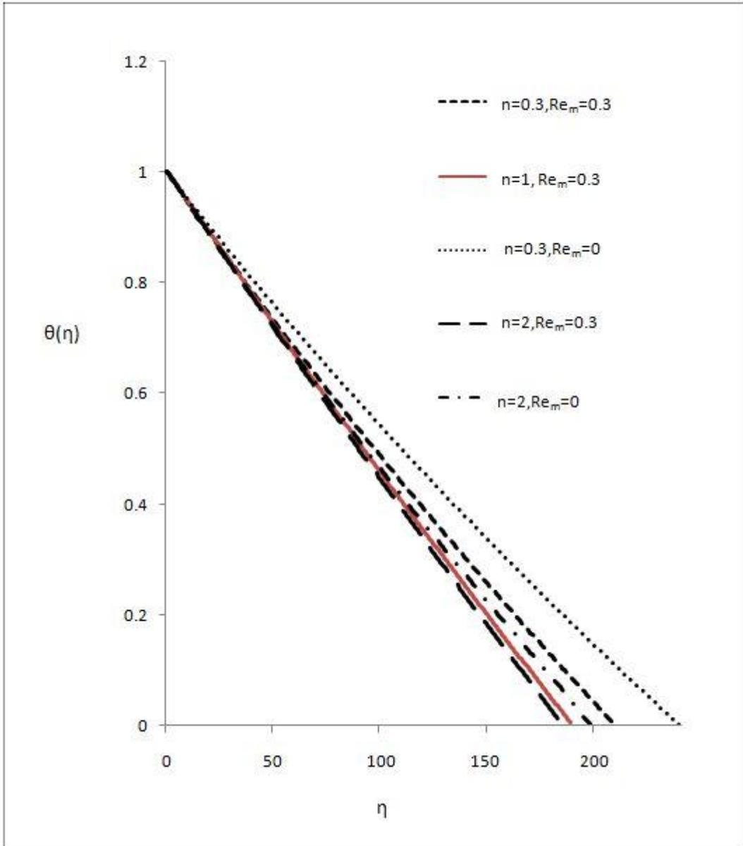
**Figure 2.8** Temperature profile against  $\eta$  for different values of  $n$  and  $Re_m$  with  $Pr = 0.02$ ,  $Ec = 0.5$  and  $\theta_r = 2.0$
