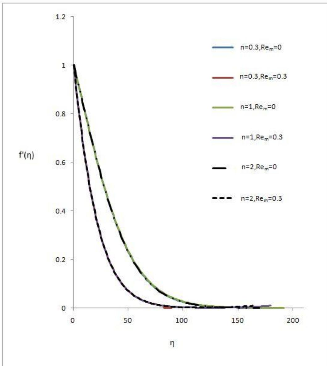
**Figure 2.4** Velocity profile against  $\eta$  for different values of  $n$  and  $Re_m$  with  $Pr = 0.02$ ,  $Ec = 0.5$  &  $\theta_r = 2.0$
