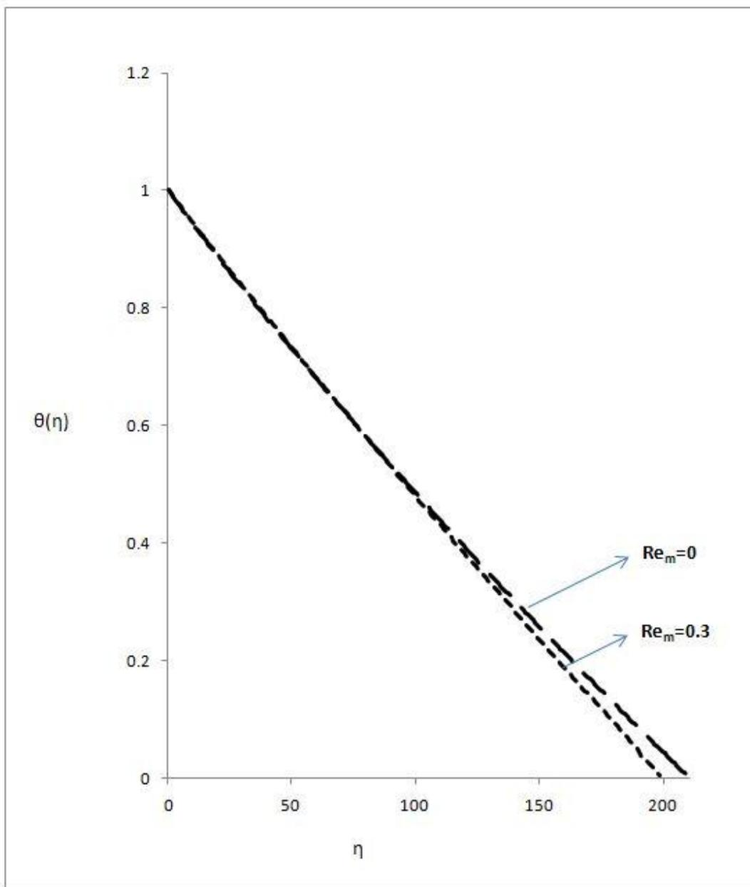
**Figure 2.9** Temperature profile against  $\eta$  for different values of  $Re_m$  with  $Pr = 0.02$ ,  $n = 0.3$  &  $Ec = 0$
