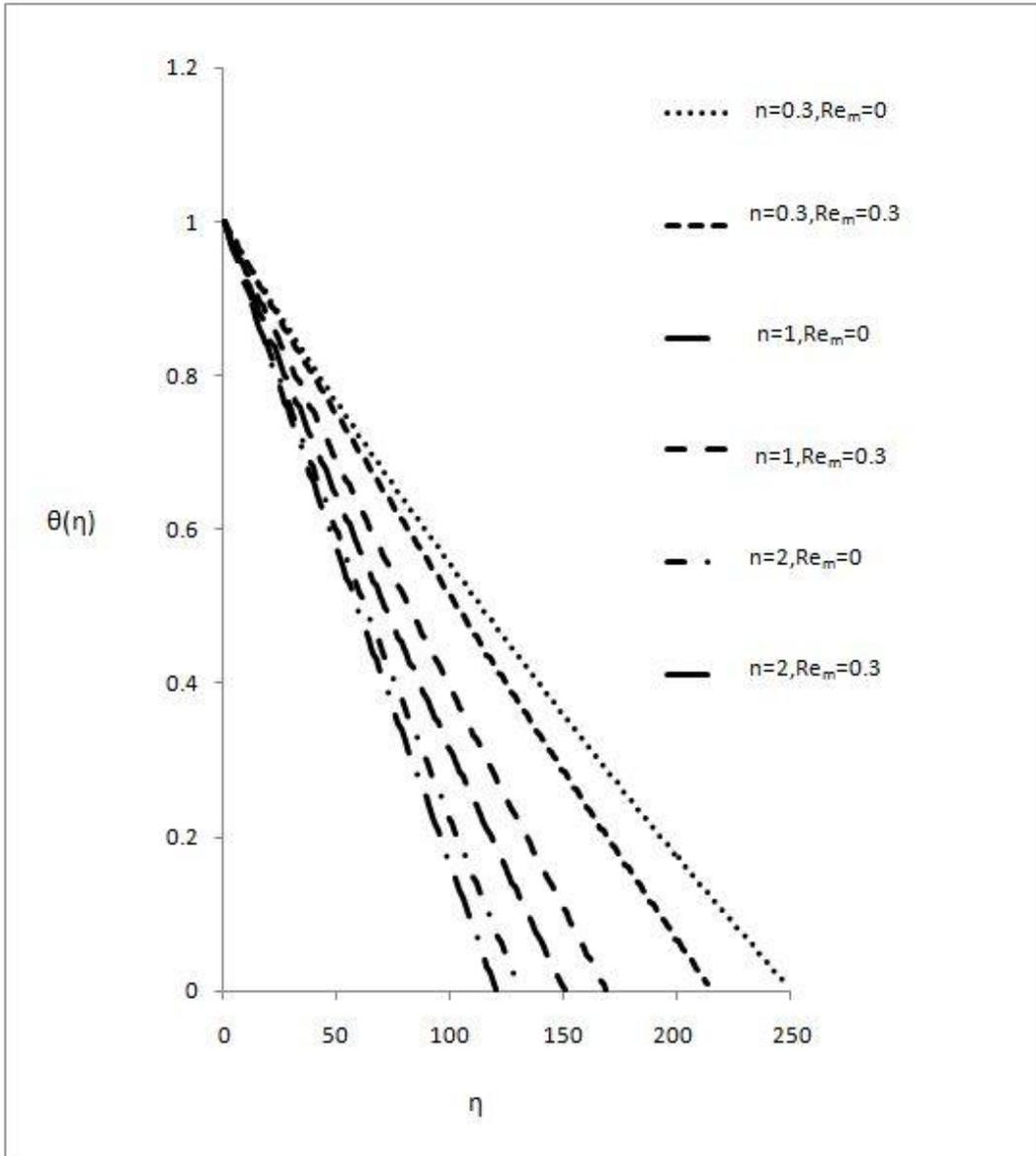
**Figure 2.7** Temperature profile against  $\eta$  for different values of  $n$  and  $Re_m$  with  $Pr = 0.02$ ,  $Ec=0.0$  &  $\theta_r=2.0$
