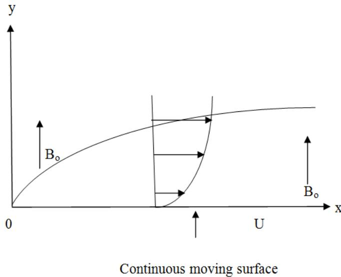
**Figure 2.1** Coordinate system for continuously moving surface
