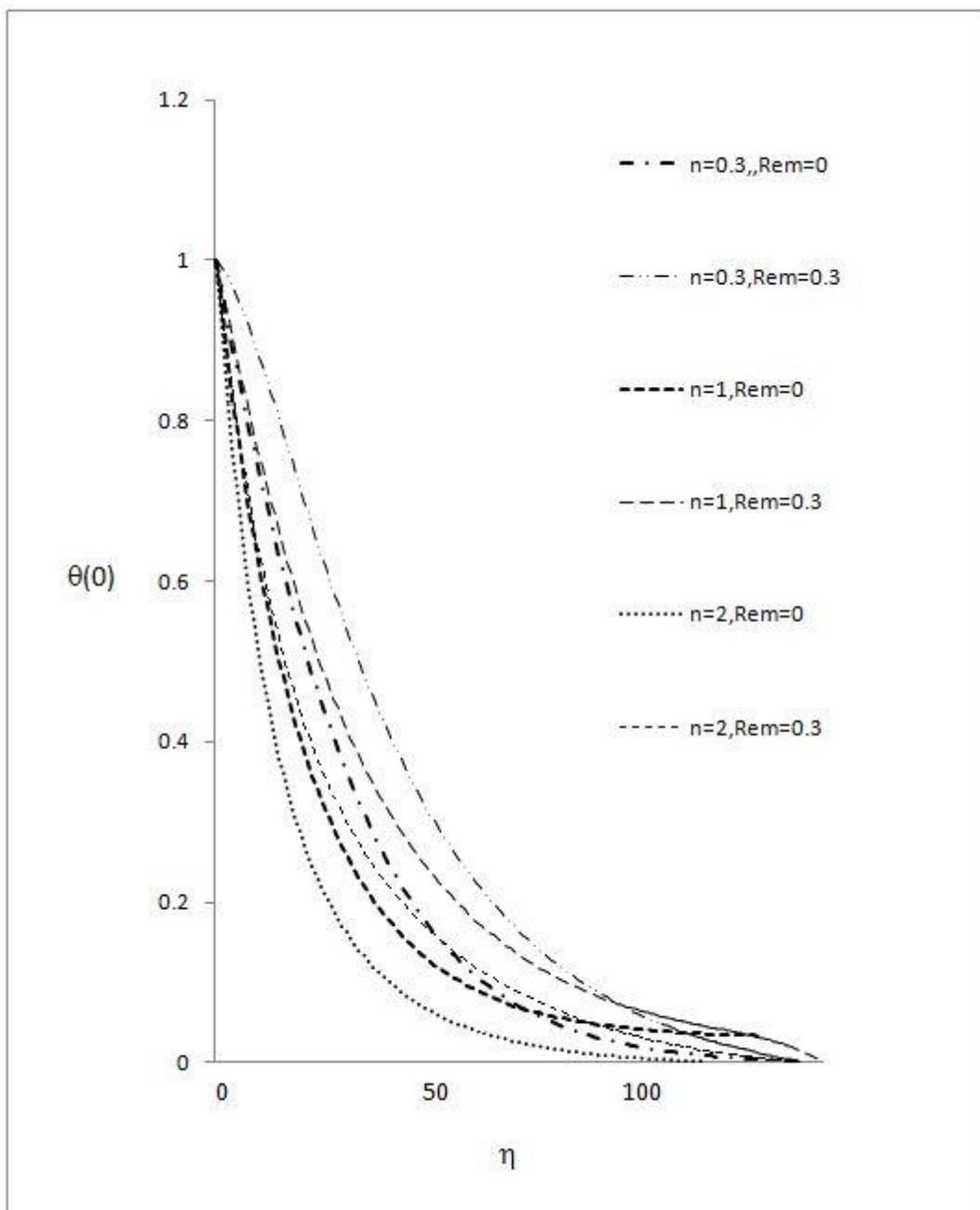
**Figure 2.6** Temperature profile against  $\eta$  for different values of  $n$  and  $Re_m$  with  $Pr = 0.02$  and  $\theta_r = 2.0$
