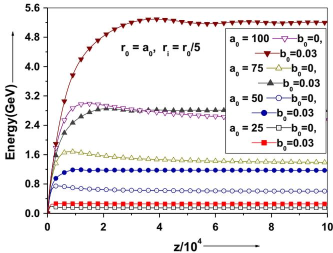
Fig. 7. Electron energy gain as a function of normalized distance in the absence and presence of a magnetic field with  $r_i = r_0/5$  and  $r_0 = a_0$  for laser intensity parameters  $a_0 = 25, 50, 75,$  and  $100$ . The other parameters are same as taken in Fig. 4.
