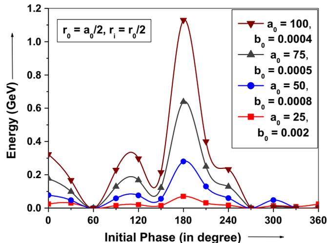
Fig. 3. Electron energy gain as a function of initial phase  $\phi_0$  with  $r_0 = a_0/2$  and  $r_i = r_0/2$  for laser intensity parameter  $a_0 = 25, 50, 75,$  and  $100$  with respective values of normalized magnetic field as obtained from Fig. 2. The other parameters are  $\tau = 200, z_L = 0, z_0 = 0,$  and  $\tau_b = 10^9$ .
