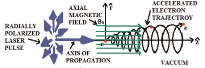
Fig. 1. A schematic showing the vacuum acceleration of electron by a Radially polarized (RP) laser pulse in the presence of axial magnetic field.
