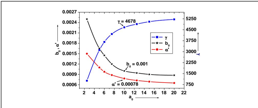
Figure 5.6. Electron energy gain  $\gamma$  calibration curve for normalized magnetic field  $b_0$ , chirping parameter  $\alpha'$  and normalized energy gain  $\gamma$  as a function of normalized intensity  $a_0$ . Rest parameters are same as taken in fig. 5.2.
