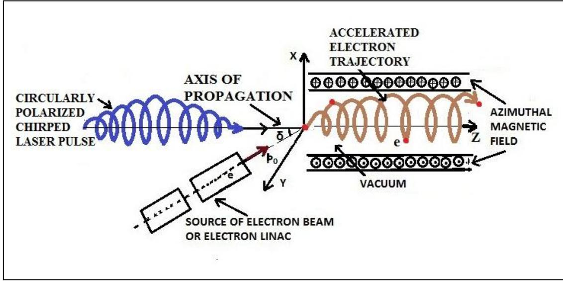
**Figure 5.1.** A schematic showing the vacuum acceleration of electron by a CP chirped laser pulse with an azimuthal magnetic field.
