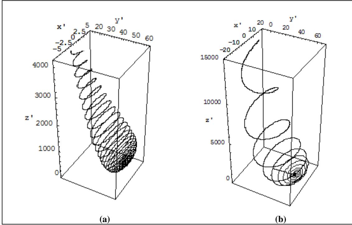
**Figure 5.2. Electron trajectory in 3D plane without and with chirping for CP laser pulse at  $a_0 = 2.5$ ,  $b_0 = 0.005$  and  $p_0' = 1$ . (a)  $\alpha' = 0$  and (b)  $\alpha' = 0.003$ . The other parameters are  $r_0' = 900$ ,  $\sigma' = 70$ ,  $\phi_0 = 0$ ,  $\delta = 10^\circ$  and  $z_0' = -300$ .**
