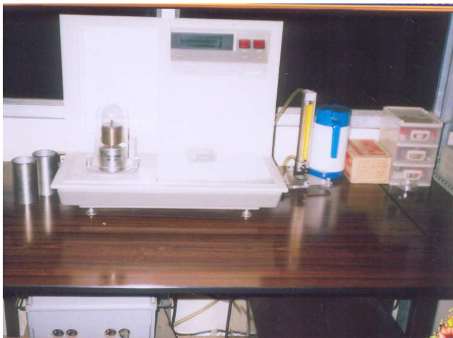
**Figure 2.2a:** DSC Setup used by the Researcher
