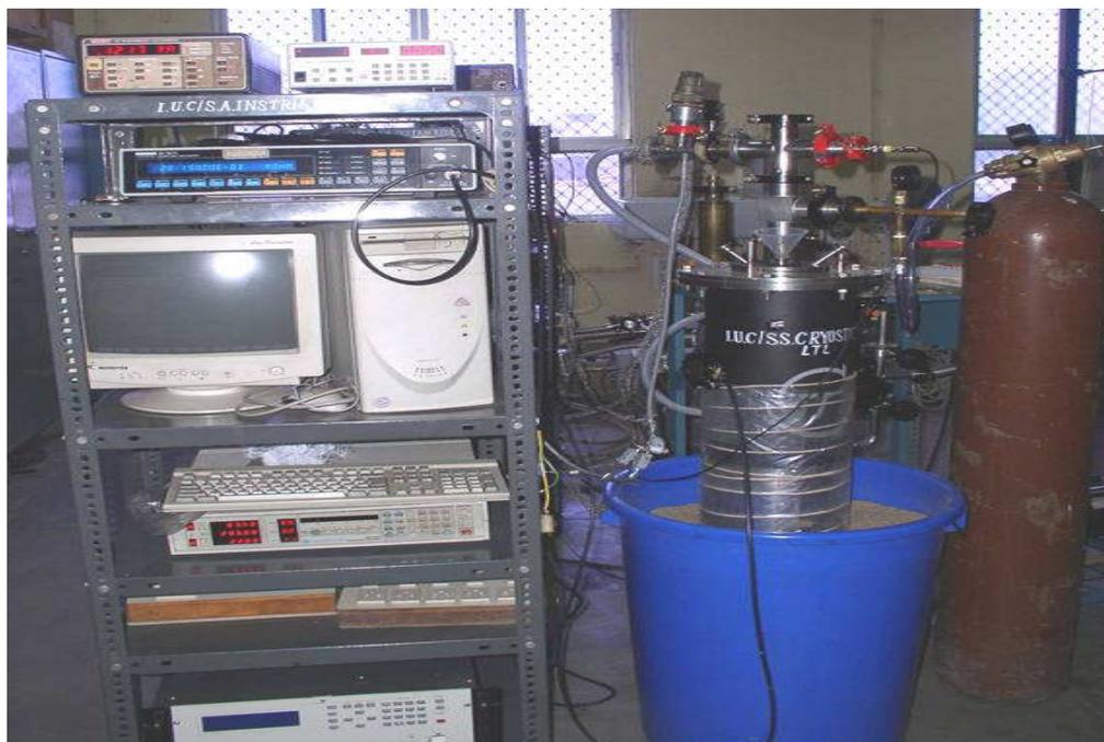
**Figure 2.6b** Low Temperature DC Electrical Resistivity Setup
