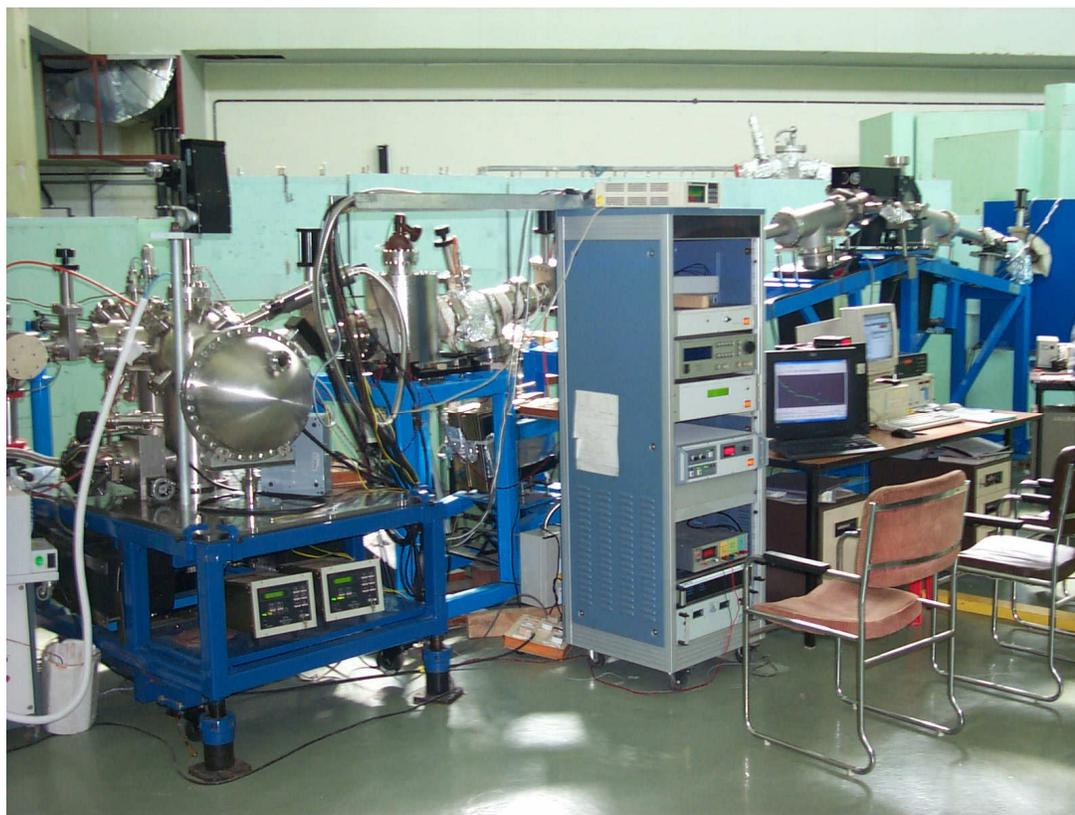
**Figure 2.5** X-Ray Photoelectron Spectrometer
