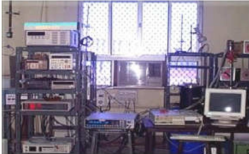
**Figure 2.6a** Low Temperature DC Electrical Resistivity Setup
