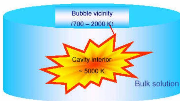
**Figure 1.4** Acoustic cavitation and reaction sites in a homogeneous liquid
