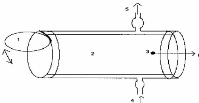
1. quartz glass window; 2. lampblack coating; 3. microphone; 4. thermostat inlet; 5. thermostat outlet; 6. PA signal to detectors.
