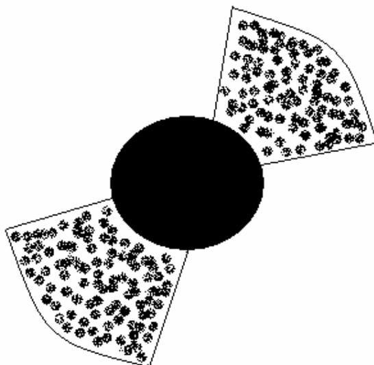
**Figure 7.3 Two segment chopper blade**
