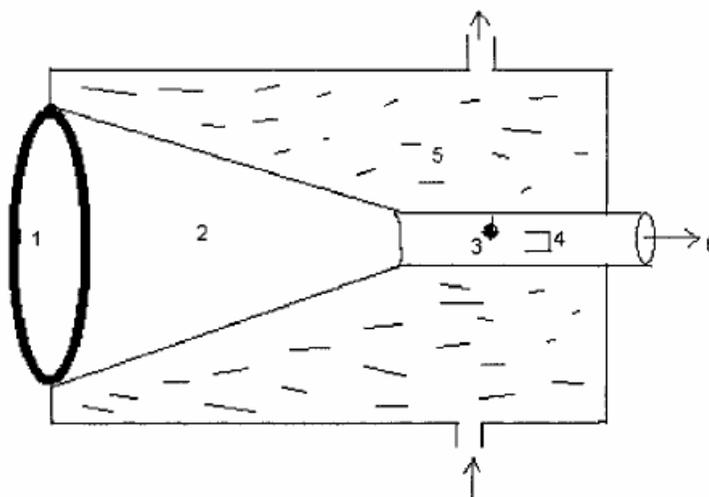
1. curved watch glass; 2. lampblack coating; 3. microphone; 4. sample holder; 5. thermostat; 6. PA signal to detectors.
