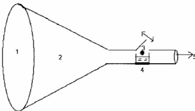
1. curved watch glass; 2. lampblack coating; 3. microphone; 4. quartz sample holder; 5. PA signal to detectors.
