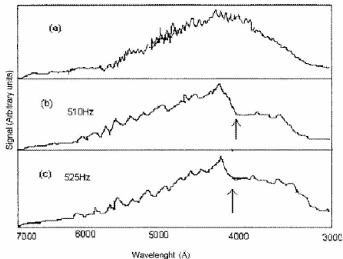
Comparison of the (a) optical and (b) photoacoustic spectra of  $\text{NO}_2$  at 10 torr (c) photoacoustic spectra of  $\text{NO}_2$  at 10 torr in the present work.
