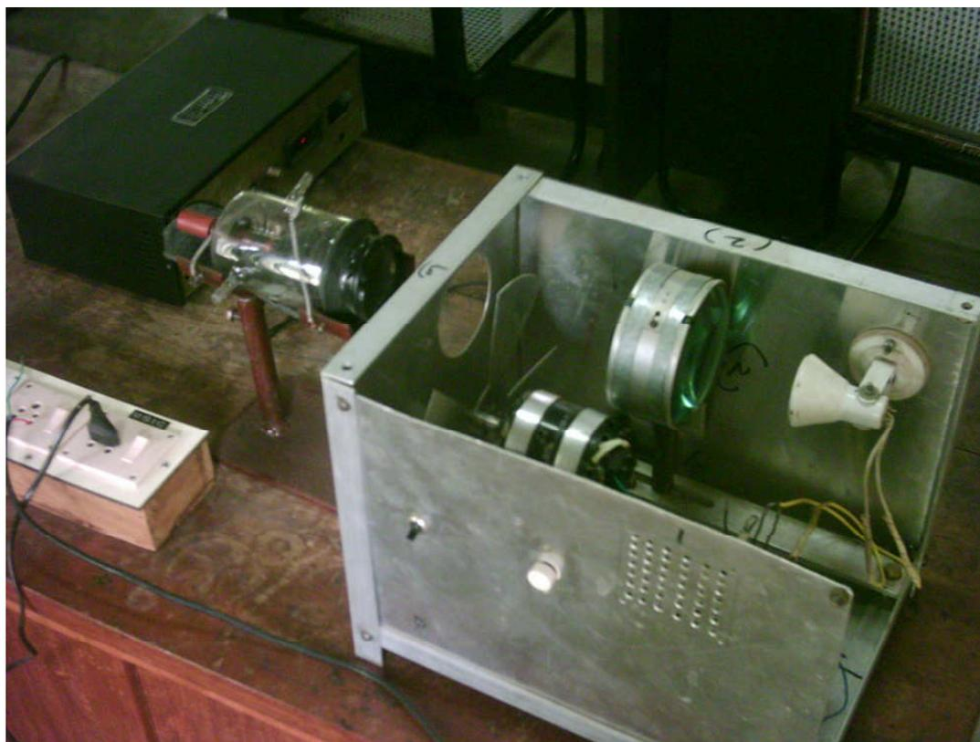
**Figure 7.2a:** Photograph of Madurai PA Spectrometer
