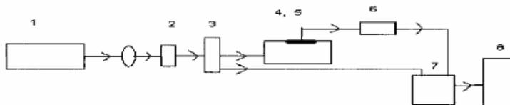
Block diagram of Madurai PA spectrometer; 1.Source; 2.Monochromator; 3. Chopper; 4. PA cell; 5. Microphone; 6. Pre-amplifier; 7. Lock-in amplifier; 8. Digital Storage Oscilloscope.
