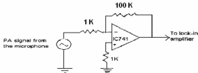
**Figure 7.7 Pre-Amplifier Circuit**
