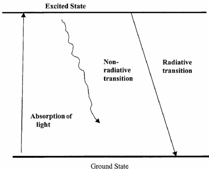
Figure 7.1 Principle of Photoacoustic Spectrum
