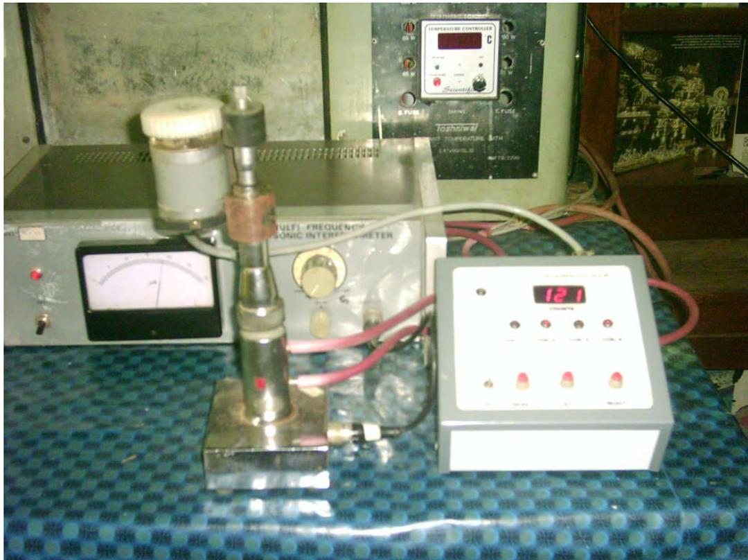
**Figure 7.9:** Photograph of digitalized micrometer screw gauge with ultrasonic interferometer.
