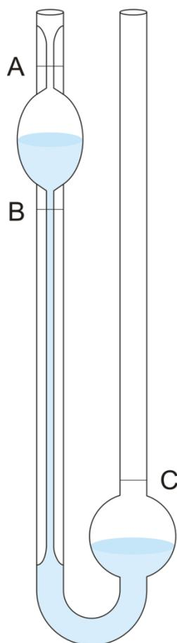
**Fig. 6.1** U-tube Viscometer
