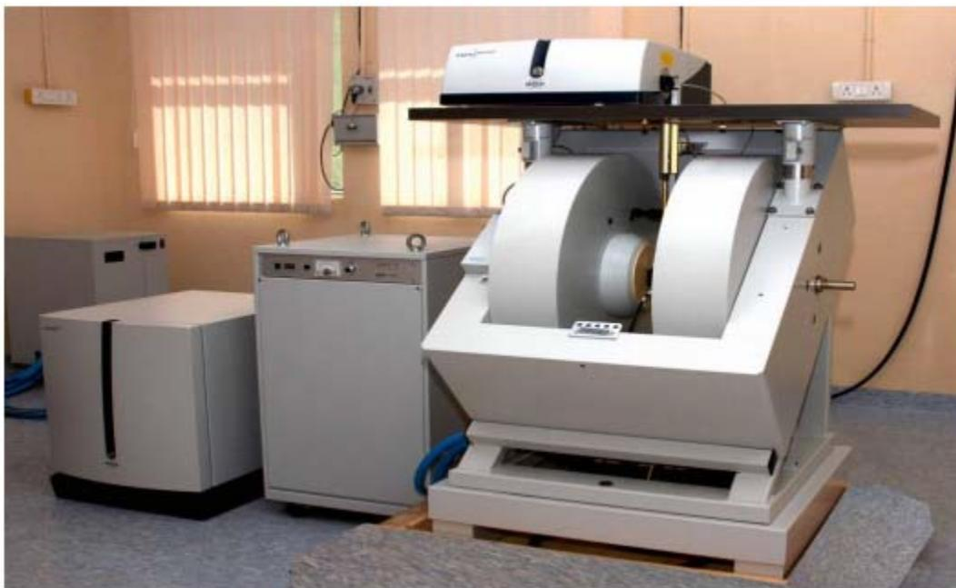
**Fig. 2.4** Photography view of X-band ESR spectrometer.
