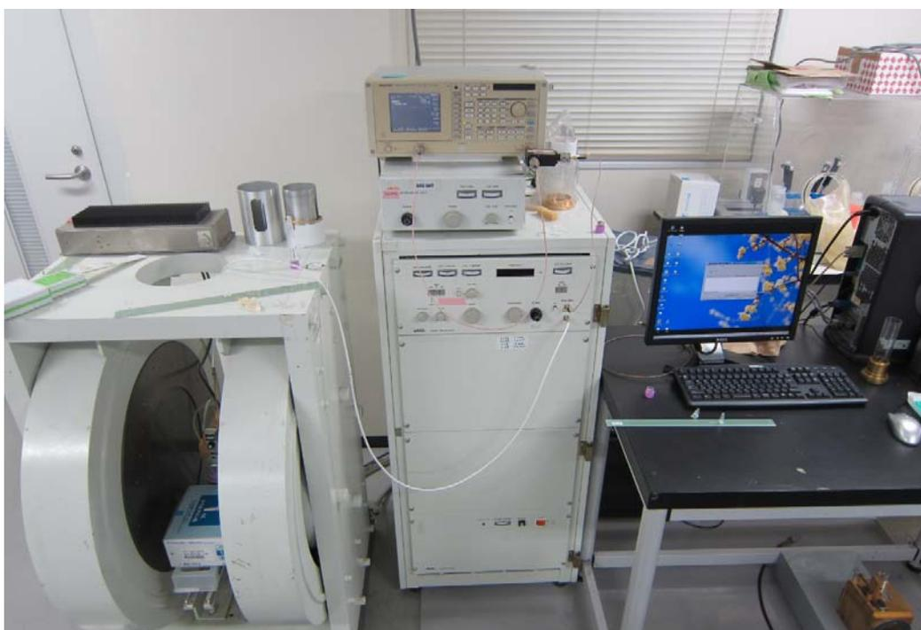
**Fig. 2.5** Photography view of L-band ESR spectrometer.
