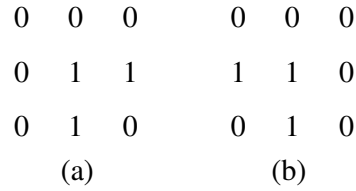
Fig. 5.2: (a) Structuring element and (b) 90^\circ rotated version of (a).
