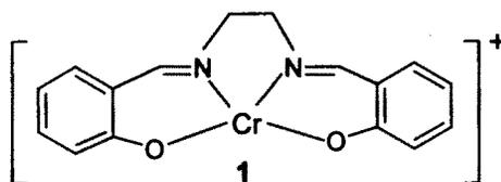
**Figure I:**  $(\text{Salen})\text{chromium}(\text{III})$  Complex
