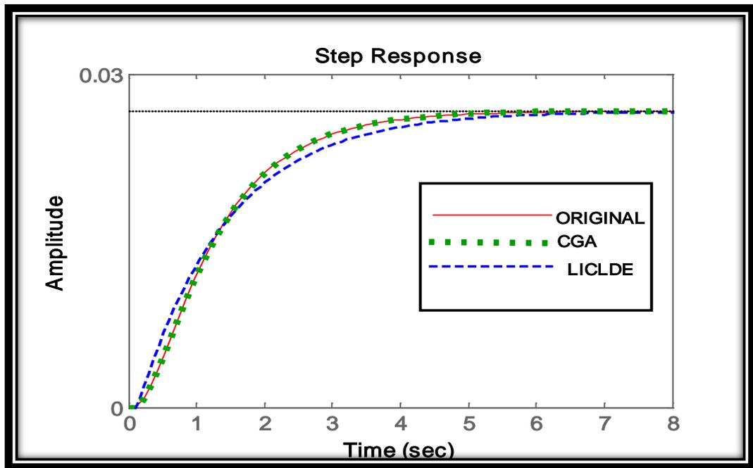
Fig. 4.5: Comparison of step responses for example 3
