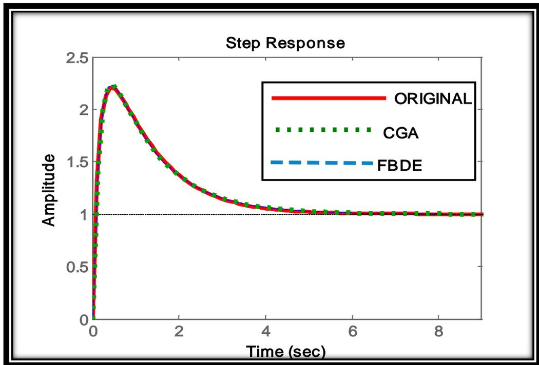
Fig. 4.1: Comparison of step responses for example 1
