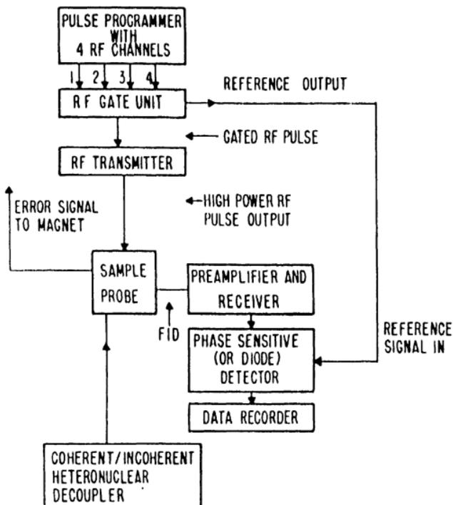
FIG 2.1 Block diagram of a versatile Bruker PC-120 NMR Process Analyser.
