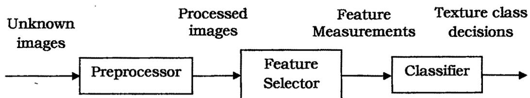
Figure 1.1: Block diagram of texture classification system.
