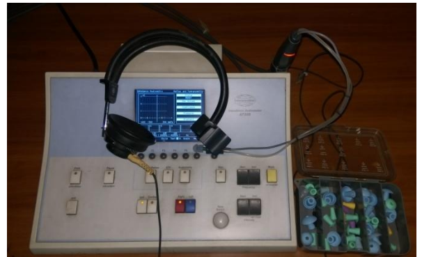
Photo 2.2-b: AT235 middle ear analyzer was used for tympanometry & MEMR using a 226 Hz probe tone.
