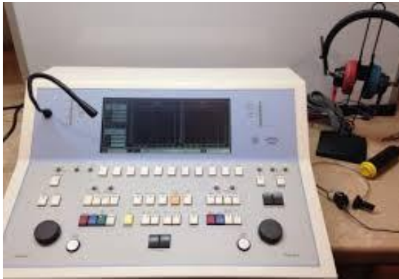
Photo 2.1-a: Showing Clinical Audiometer AC – 40 used for data collection for Pure Tone audiometry, Free field audiometry, Play audiometry and Speech audiometry.
