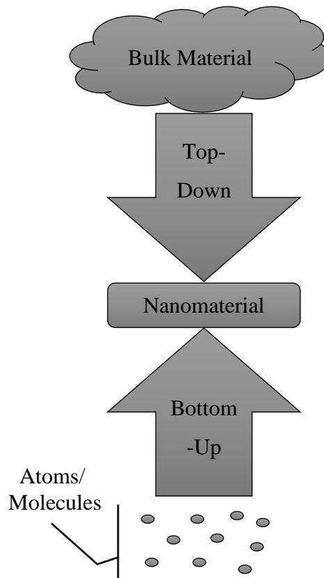
Figure 4 Basic Synthetic Approaches of Nanomaterials
