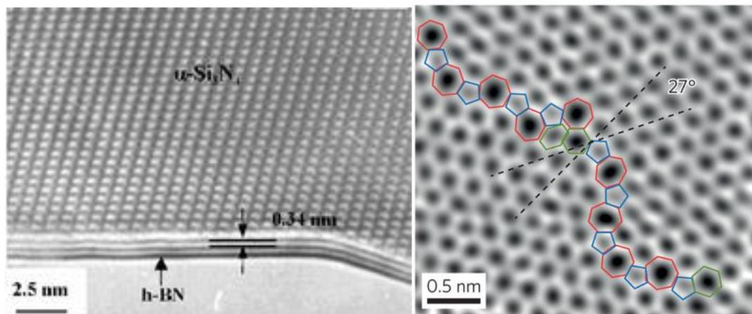
Figure 3 Nano-Film<sup>18</sup> (2D) of  $\text{Si}_3\text{N}_4$  (Left), Polycrystalline (3D) graphene grains with two lattice orientations<sup>19</sup> (Right)
