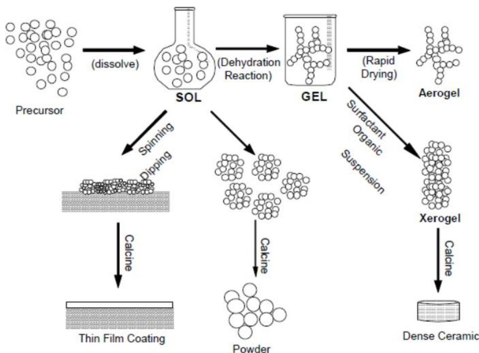
Figure 5 schematic representation of Sol-Gel Method<sup>21</sup>
