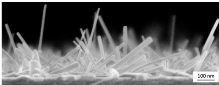
Figure 2 Nanowires (1D) of Tungsten oxide<sup>17</sup>
