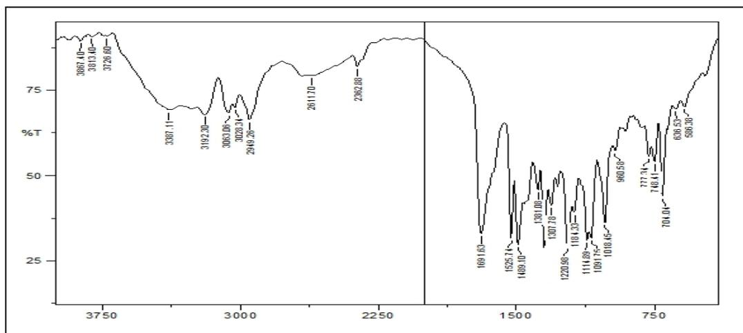
**Fig 3.2.** FTIR spectra of lercanidipine hydrochloride.
