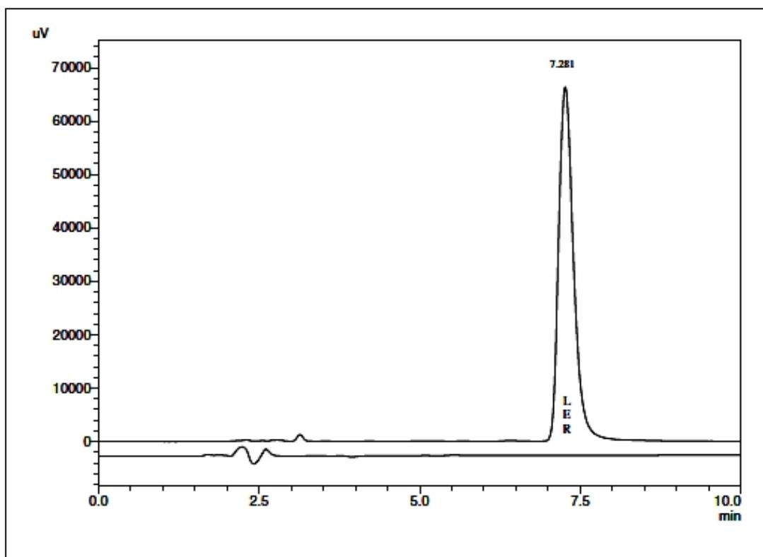
**Fig. 3.3.** Typical chromatogram of lercanidipine hydrochloride.
