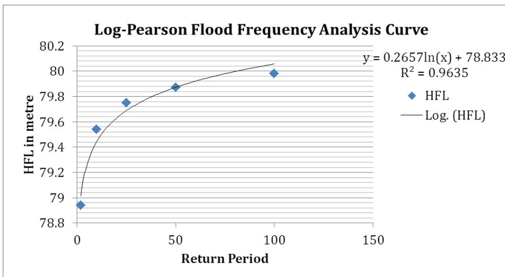
**Fig 8.5: Flood Frequency Analysis Curve**
