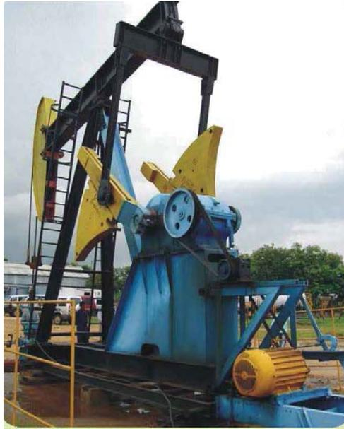
**Figure 1.10: Sucker Rod Pump at Well Head as EOR Method**
