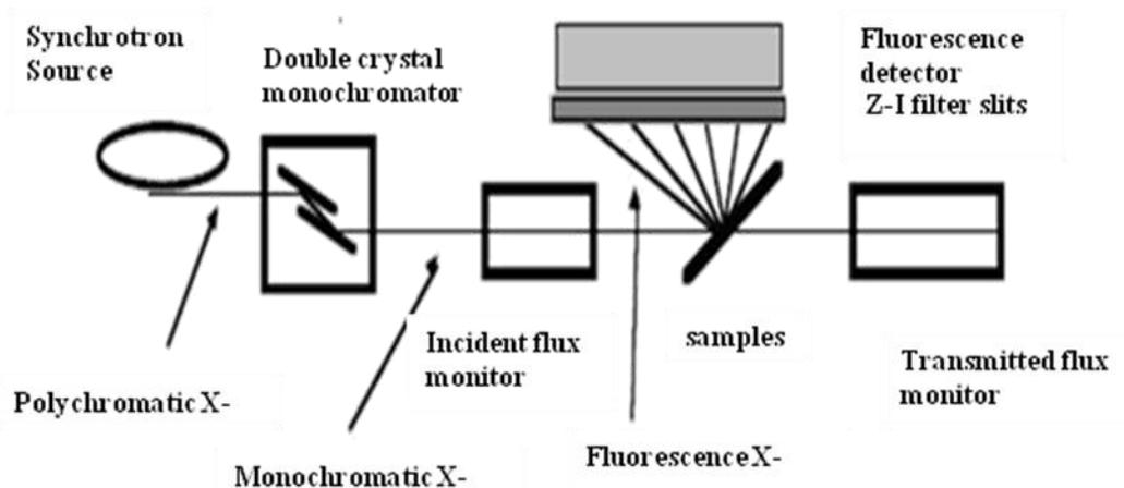
**Figure 1-10 Schematic of XAFS experiment**
