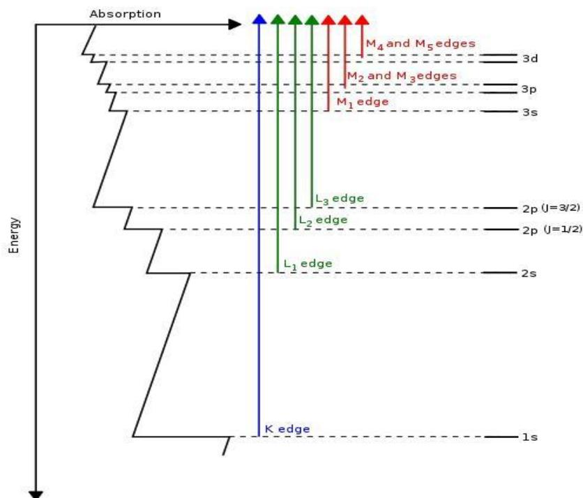
**Figure 1-6 The relationship between the X-ray absorption edges and the corresponding excitation of core electrons.**
