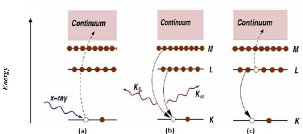
**Figure 1-13 The fundamental processes which contribute to XANES spectra**
