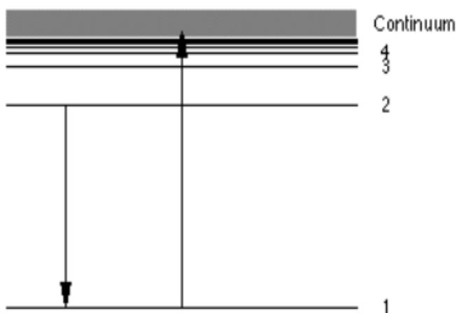
**Figure 1-9 Excitation of photoelectron from 1S state to continuum.**
