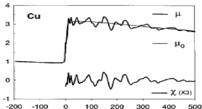
**Figure 1-8 The relationship between the X-ray absorption coefficient  $\mu(E)$ , the smooth atomic like background  $\mu_0(E)$ , and  $\chi(E)$  for a Cu K edge.**
