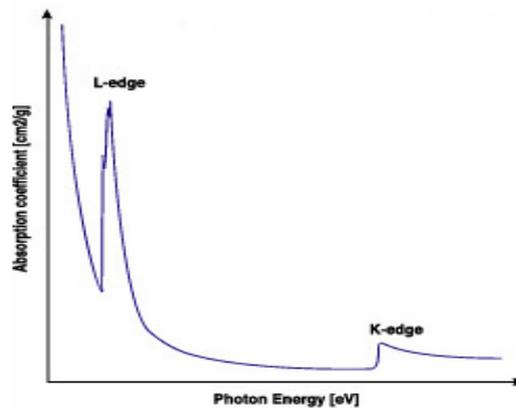
**Figure 1-5 X-ray absorption coefficient vs photon energy**
