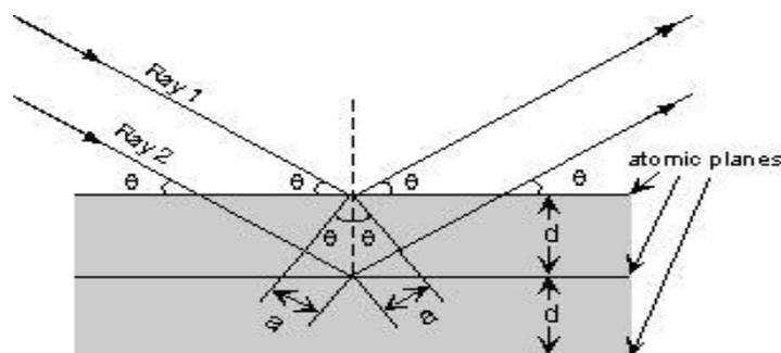
**Figure 1-17 Bragg's diffraction**
