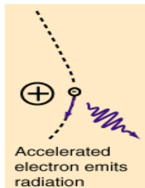
Figure 1-2 Bremsstrahlung X-rays
