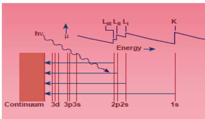
**Figure 1-12 XAS Edge result from core ionization**
