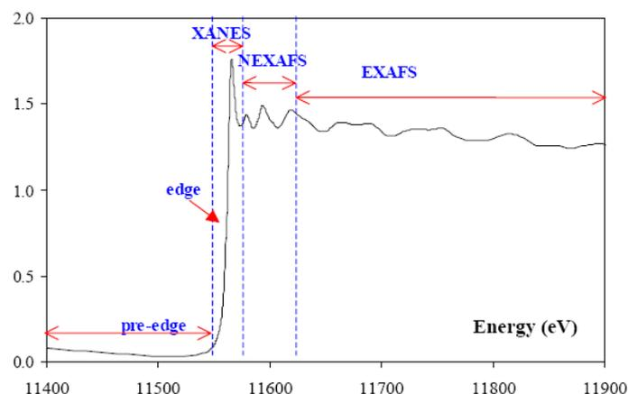
**Figure 1-7 The normalized K-absorption spectrum of copper metal showing the pre-absorption, XANES and EXAFS regions**
