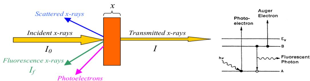
**Figure 1-4 Absorption processes for X-rays**
