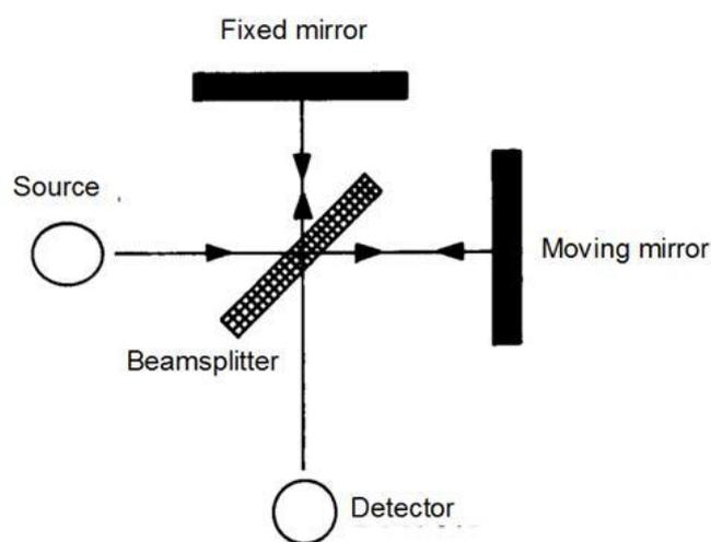
Figure 1-16 Schematic diagram of a Michelson Interferometer.
