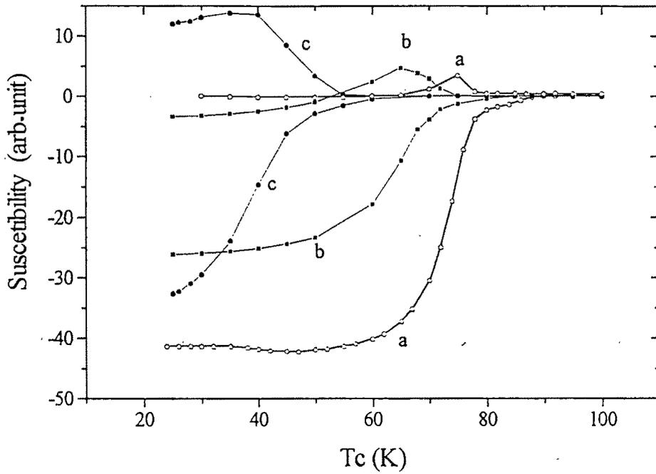
Fig.V.2.AC magnetic susceptibility variation with temperature in  $\text{YBa}_2\text{Cu}_{3-x}\text{Ag}_x\text{O}_{7-y}$  samples. (a)  $x = 0, y = .072$ , (b)  $x = 0.06, y = 0.092$ , (c)  $x = 0.12, y = 0.230$ .
