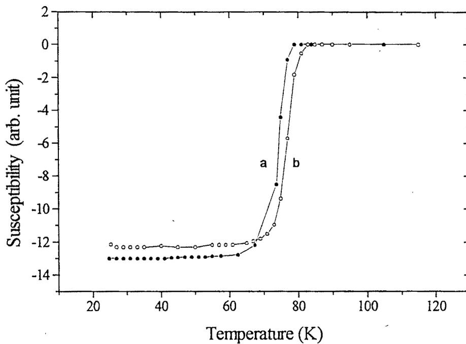
Fig.V.7. AC magnetic susceptibility variation with temperature in  $\text{YBa}_2\text{Cu}_{3-x}\text{Ag}_x\text{O}_{7-y}$  samples with  $x = 0.12$  (a) quenched from 500 C (b) quenched from 500 C and annealed for 2hrs.
