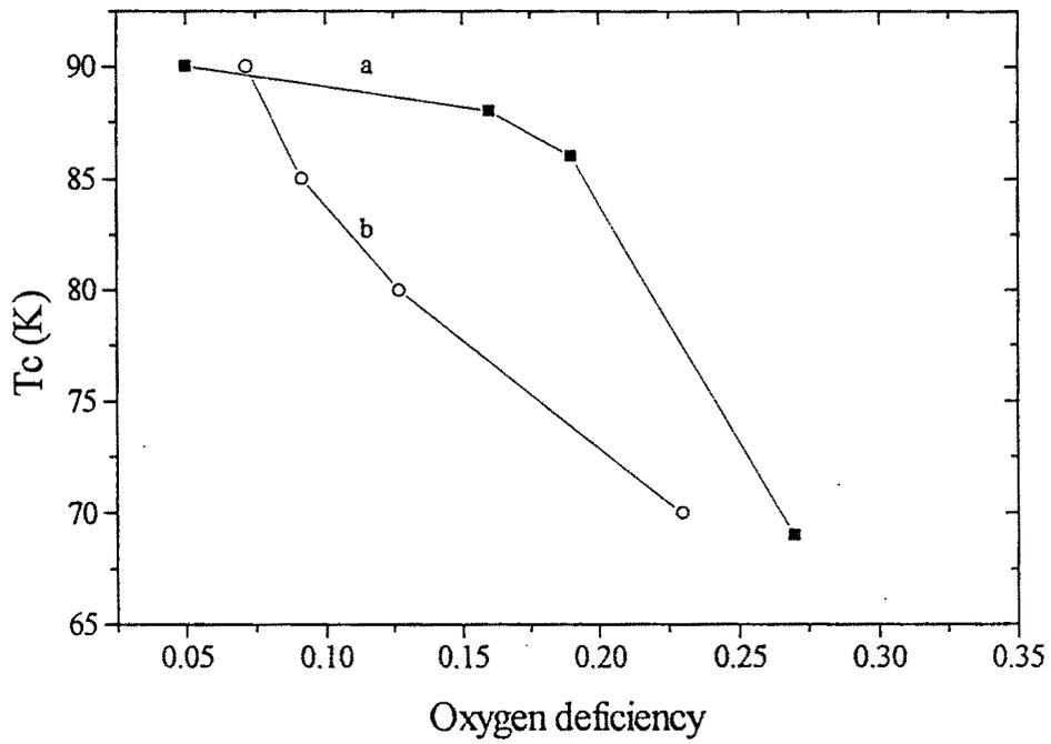
Fig.V.5. Transition temperature ( $T_c$ ) dependence on oxygen deficiency in (a)  $\text{YBa}_2\text{Cu}_3\text{O}_{7-y}$  and (b)  $\text{YBa}_2\text{Cu}_{3-x}\text{Ag}_x\text{O}_{7-y}$  samples with  $x = 0.12$
