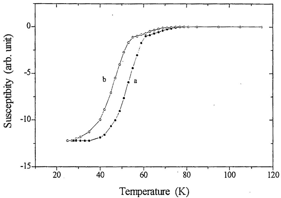
Fig.V.6. AC magnetic susceptibility variation with temperature in  $\text{YBa}_2\text{Cu}_3\text{O}_{7-y}$  samples (a) quenched from 500 C (b) quenched from 500 C and annealed for 2hrs.
