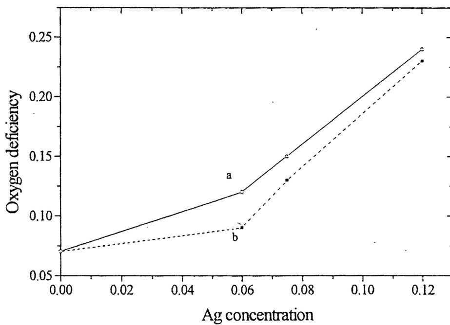
Fig.V.3. Variation of oxygen deficiency in  $\text{YBa}_2\text{Cu}_{3-x}\text{Ag}_x\text{O}_{7-y}$  samples
