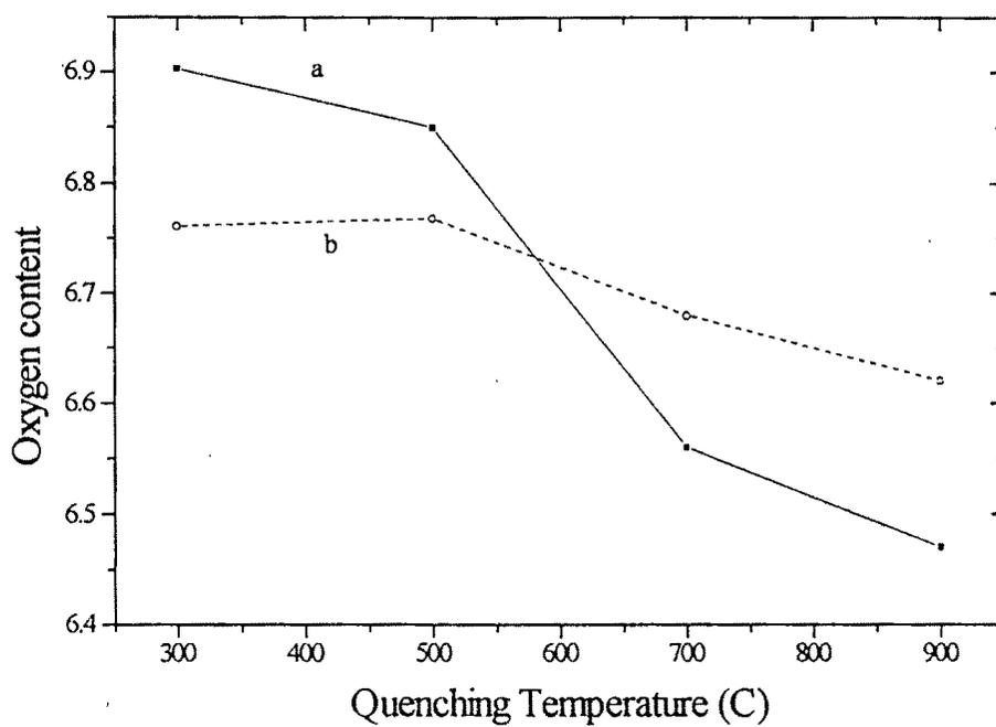
Fig.V.8. Variation of oxygen content with quenching temperature in (a)  $\text{YBa}_2\text{Cu}_3\text{O}_{7-y}$  sample (b)  $\text{YBa}_2\text{Cu}_{3-x}\text{Ag}_x\text{O}_{7-y}$  sample with  $x = 0.12$
