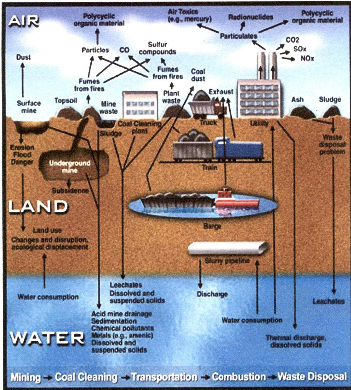
Fig 1 : Schematic presentation of the Mining activities and associated emissions
