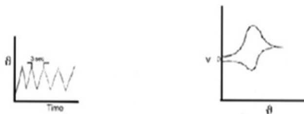
Fig:2: a) Type of Wave Used in Cyclic Voltammetry b) Type of iv curve obtained using Cyclic Voltammetry
