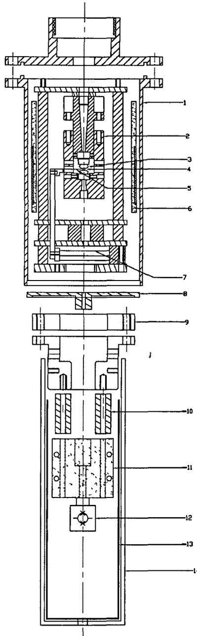
[1. Exchange gas chamber, 2. Piston-Cylinder type DAC, 3. Diamond, 4. Sample, 5. SC pick-up coil (Gradiometer type), 6. Magnetic Solenoid, 7. Bi-morph Piezoelectric actuators, 8. OFHC Copper bottom, 9. SQUID Assembly holder - Mat. Brass, 10. OFHC copper tube, 11. SQUID electronics board holder - Mat. Hylem, 12. dc SQUID, 13. Pb shield, 14. Cryoperm shield]
