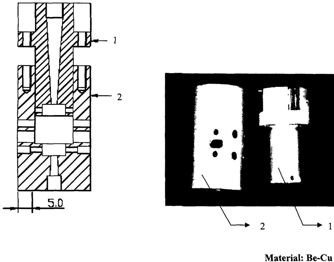
Figure 5.1 Schematic diagram of piston-cylinder type diamond anvil cell
