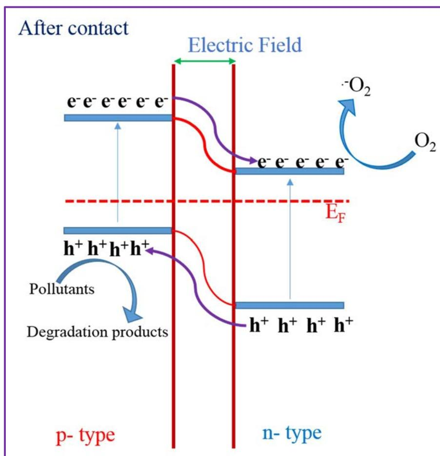
**Fig. 1.9:** Electron-hole pair separation in p-n heterojunction.
