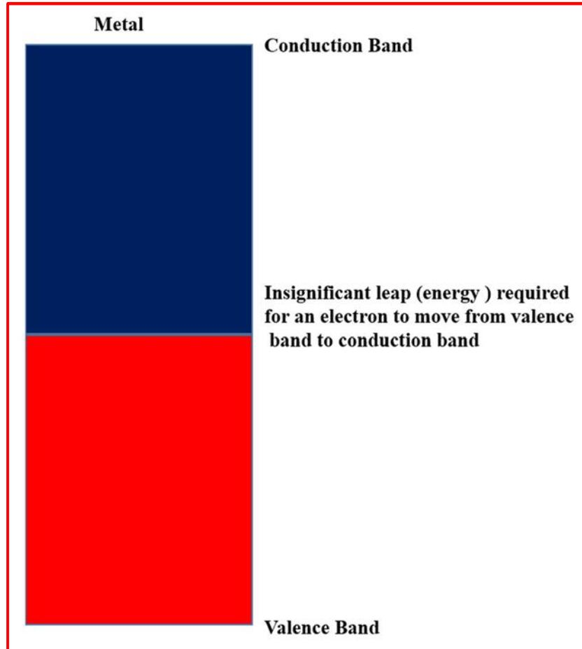
**Fig. 1.2:** Energy band diagram of metals.
