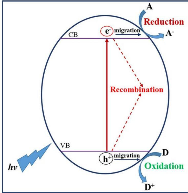
**Fig. 1.5:** Schematic illustration of principle of photocatalysis.
