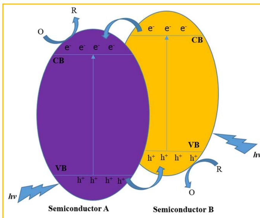
**Fig. 1.10:** Schematic diagram showing the energy band structure and electron-hole pair separation in S-S nanocomposite system.
