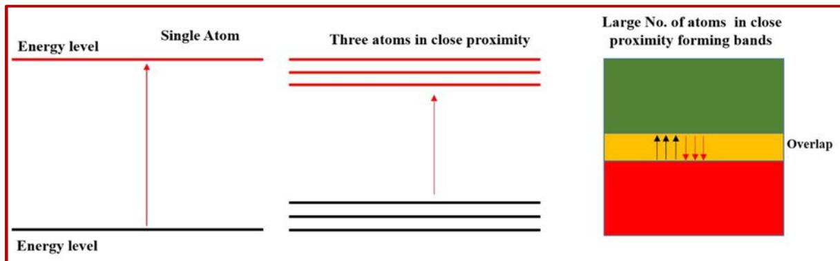
**Fig. 1.1:** Schematic representation showing energy level spacing in single atom, three atoms, and multitude of atoms.
