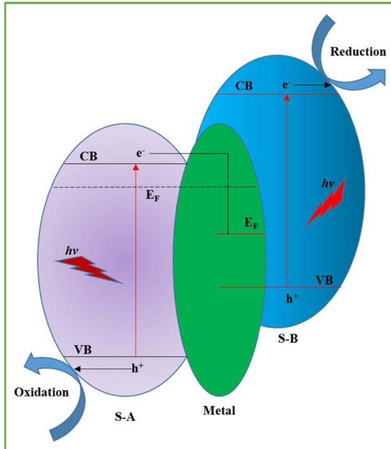
**Fig. 1.11:** Schematic diagram showing electron hole pair separation in multicomponent heterojunction.
