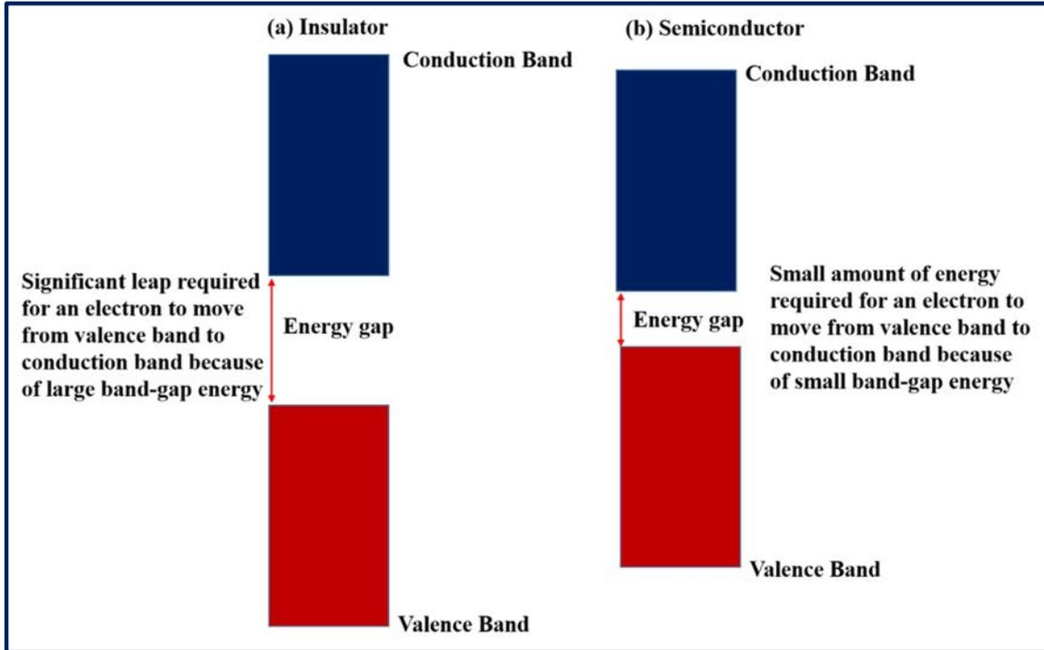
**Fig. 1.3:** Energy band separation in insulators and semiconductors.
