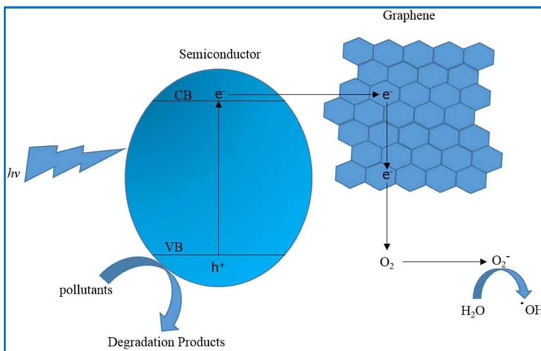
**Fig. 1.8:** Schematic diagram showing Semiconductor-graphene heterojunction.
