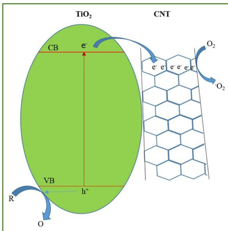
**Fig. 1.7:** Mechanism for TiO<sub>2</sub>/CNT heterojunction.
