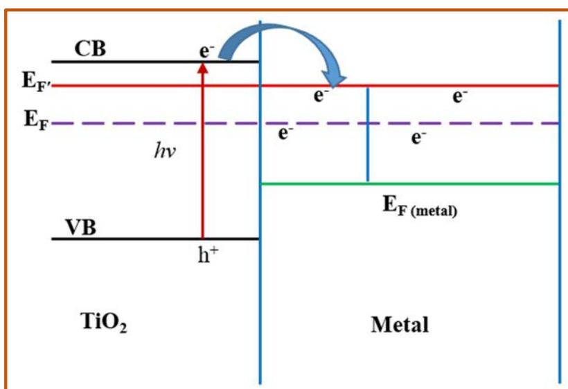
**Fig. 1.6:** Fermi level equilibration in Au/TiO<sub>2</sub> semiconductor nanoparticle.  $E_F$  and  $E_{F'}$  refer to the Fermi level of TiO<sub>2</sub> before and after equilibration.
