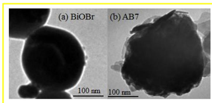
**Fig. 4.4:** TEM images of the samples: (a) BiOBr, (b) AB7.
