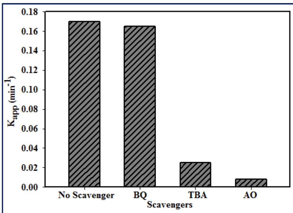
**Fig. 4.12:** Effect of scavengers on decolourization of RhB over AB7; BQ=Benzoquinone, TBA=tert-butylalcohol, AO=ammonium oxalate.
