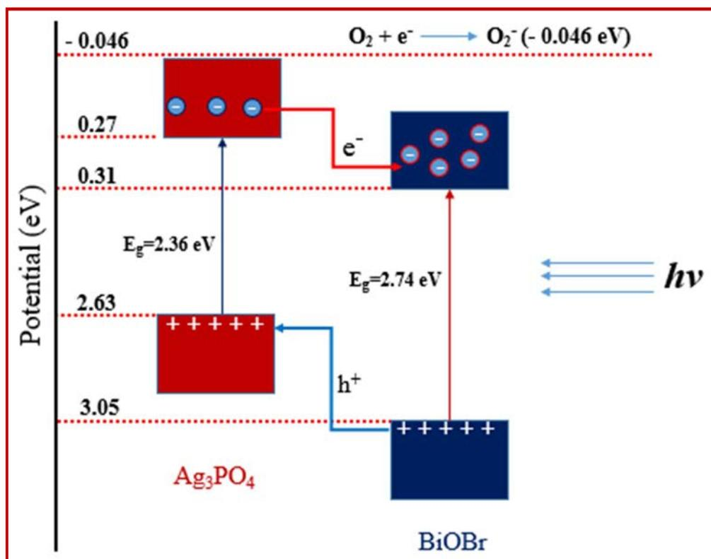
**Fig. 4.14:** Schematic diagram of electron-hole pair separation and the possible reaction mechanism over Ag<sub>3</sub>PO<sub>4</sub>/BiOBr photocatalyst under visible light irradiation.
