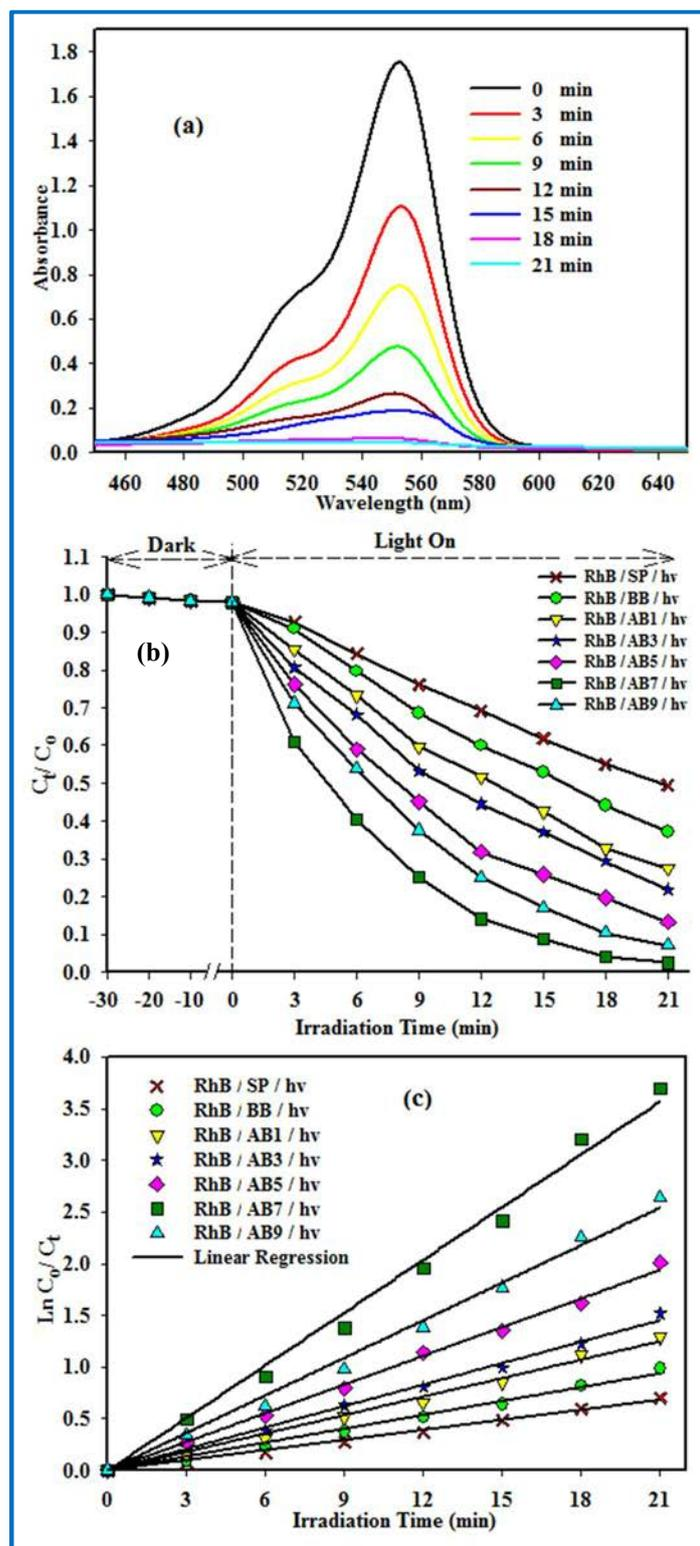
**Fig. 4.10:** (a) Change in UV-vis spectra of RhB aqueous suspension in the presence of AB7 at different irradiation times, (b) Change in concentration ( $C_t/C_0$ ) of RhB in the presence of  $Ag_3PO_4$ , BiOBr, and  $Ag_3PO_4/BiOBr$  hybrids under visible light, and (c)  $\ln(C_0/C_t)$  versus irradiation time for different catalysts.
