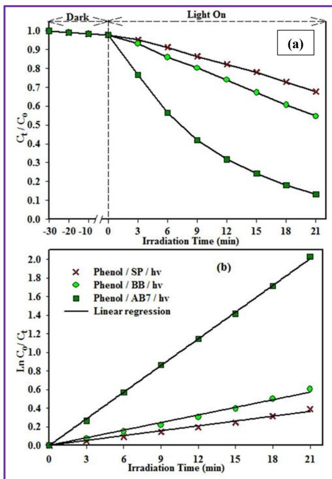
**Fig. 4.13:** (a) Change in concentration ( $C_t/C_0$ ) of phenol in the presence of BiOBr,  $Ag_3PO_4$  and AB7 (b) Phenol degradation curves of  $\ln(C_0/C_t)$  versus irradiation time for BiOBr,  $Ag_3PO_4$  and AB7.
