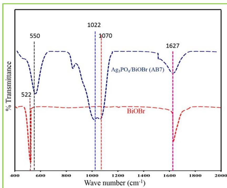
**Fig. 4.5:** FTIR spectra of BiOBr and AB7.
