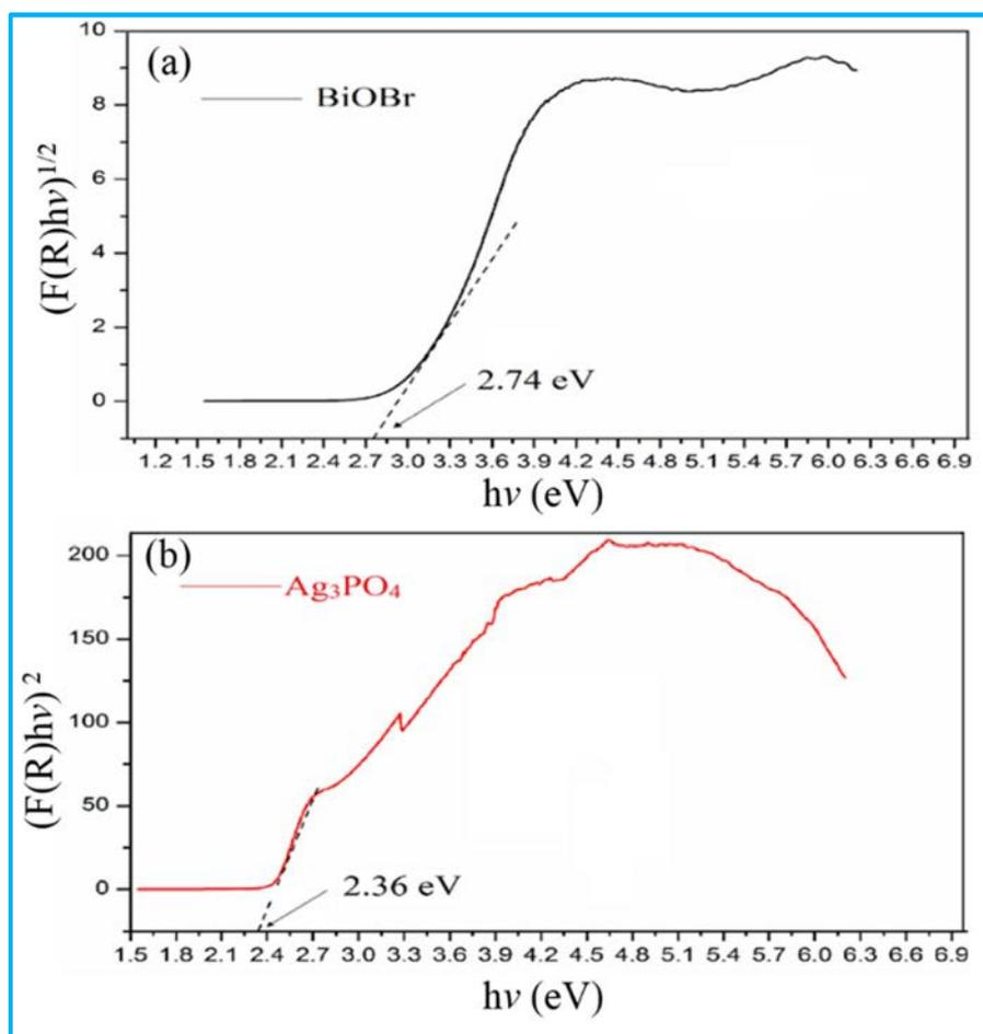
Fig. 4.8: (a) Plot of  $(F(R).hv)^{1/2}$  versus energy ( $h\nu$ ) for the band gap energy of BiOBr, and (b)  $(F(R).hv)^2$  versus energy ( $h\nu$ ) for  $\text{Ag}_3\text{PO}_4$ .
