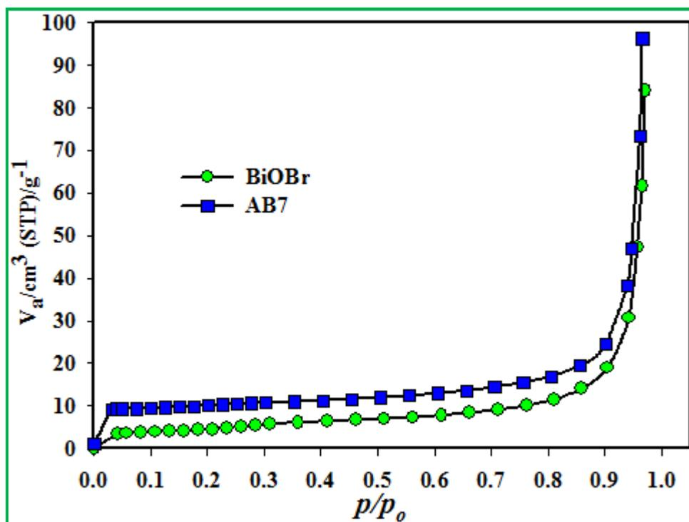
Fig. 4.6: Nitrogen adsorption–desorption isotherms for BiOBr and AB7.
