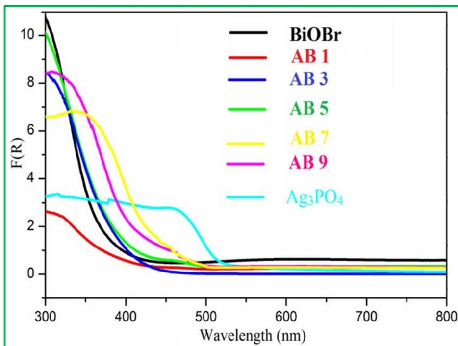
Fig. 4.7: DRS of BiOBr and  $\text{Ag}_3\text{PO}_4/\text{BiOBr}$  hybrids.
