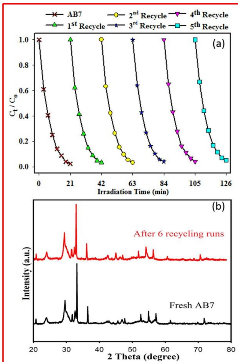
**Fig. 4.15:** (a) Cycling runs of AB7 for decolourization of RhB under visible light, (b) XRD patterns of Fresh AB7 and used AB7 after 6 recycling runs.
