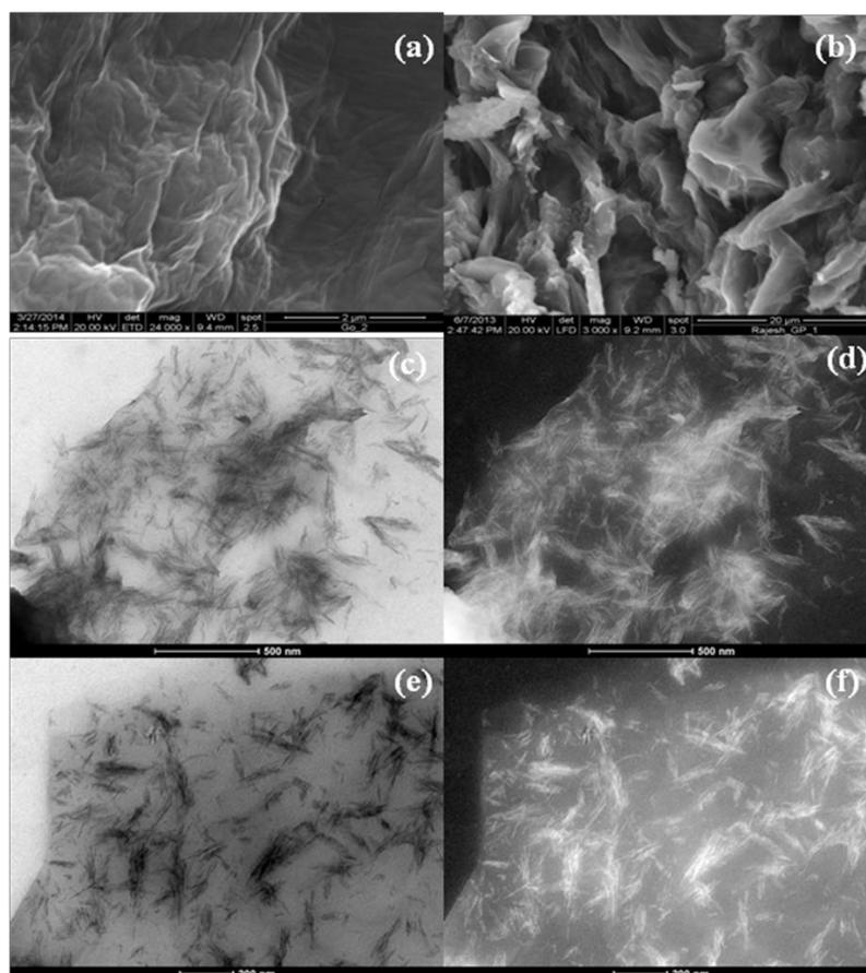
**Figure A.3** SEM images of (a) GO and (b) GO-HAP nanocomposites, **Figure A.3** (c) and (e) are bright field images of GO-HAP nanocomposites and the **Figure A.3** (d) and (f) are its corresponding dark field images
