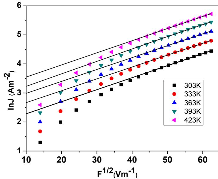
**Figure A.7** Plot between  $\ln J$  and  $F^{1/2}$  for I-V data in the high field region
