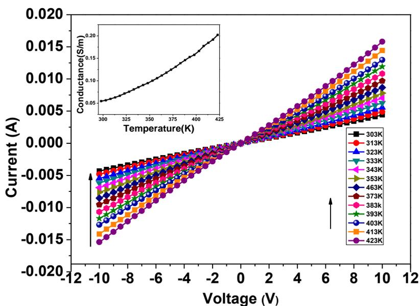
**Figure A.6** Temperature-dependent I-V characteristics of the GO-HAP nanocomposites measured in the range of 300 K - 473 K and inset figure shows the temperature versus conductivity graph for GO-HAP nanocomposites
