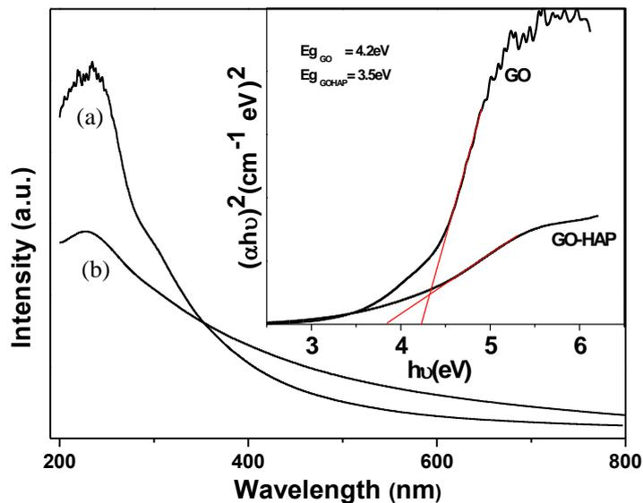
**Figure A.5** UV-Visible absorbance spectra of (a) GO and (b) GO-HAP nanocomposite. Inset figure shows the plot between  $(\alpha h\nu)^2$  Vs  $h\nu$  graph for the GO and GO-HAP nanocomposite
