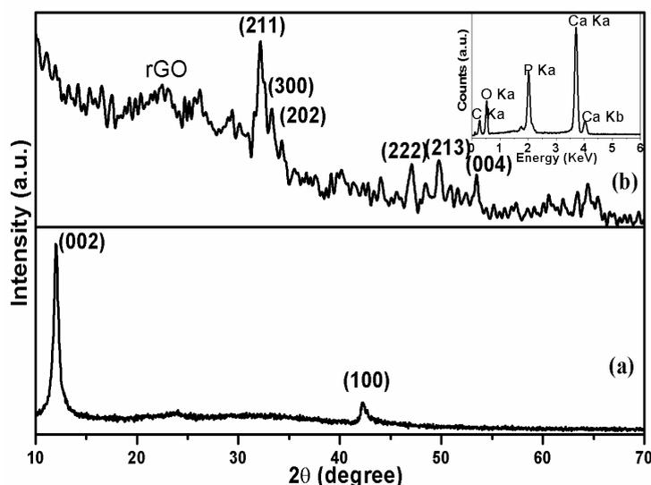
**Figure A.2** X-ray diffraction patterns of (a) GO, (b) GO-HAP composites and inset Figure A.2b shows the EDS spectrum of GO-HAP nanocomposite
