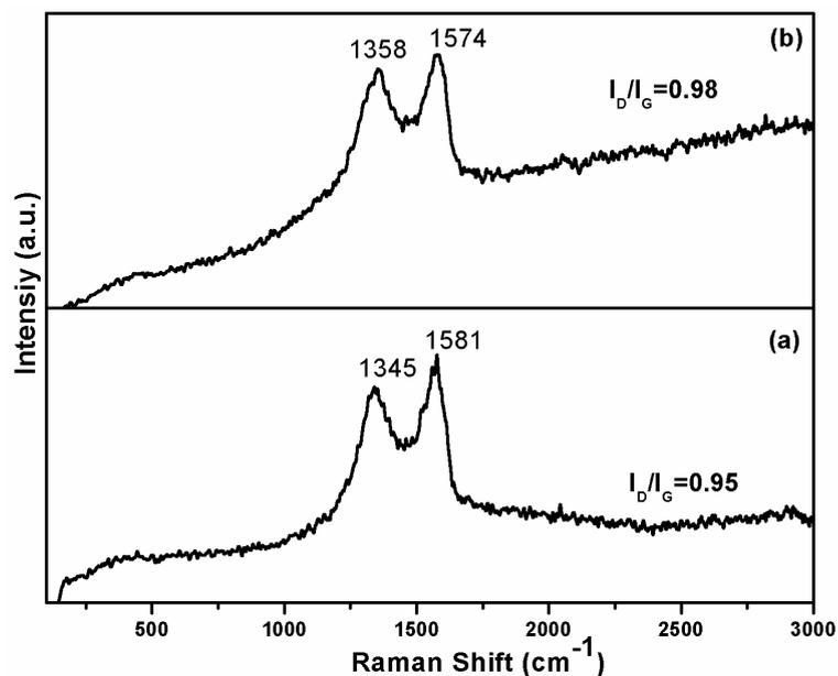
**Figure A.4** Raman spectrum of (a) GO and (b) GO-HAP nanocomposite
