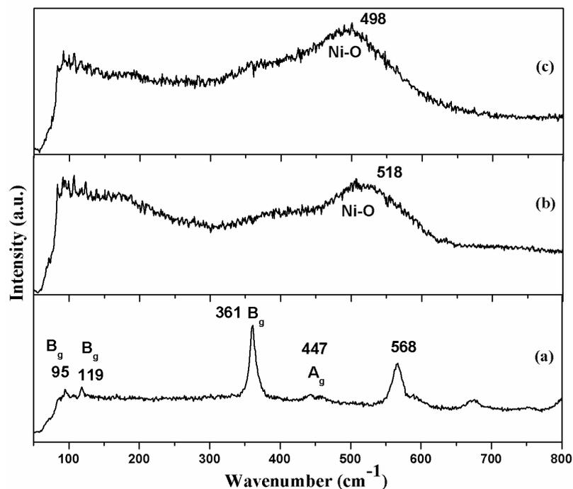
**Figure 8.2** Raman spectra of (a)  $\text{Gd}_2\text{O}_3$ , (b) NiO and (c)  $\text{Gd}_2\text{O}_3/\text{NiO}$  NPs
