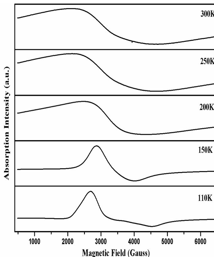
**Figure 8.5** EPR spectra for  $Gd_2O_3/NiO$  CSNPs obtained at low temperatures of 300K-110K
