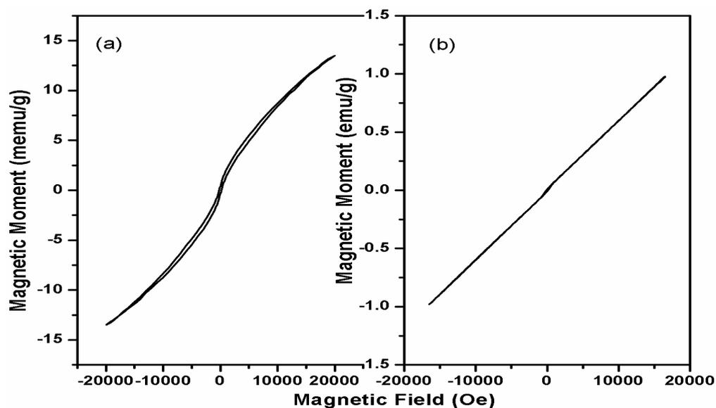
**Figure 8.4** Room temperature hysteresis curves obtained for (a) NiO and (b)  $Gd_2O_3/NiO$  CSNPs
