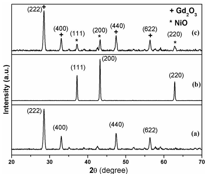
**Figure 8.1** X-ray diffraction patterns obtained for (a)  $\text{Gd}_2\text{O}_3$ , (b) NiO and (c)  $\text{Gd}_2\text{O}_3/\text{NiO}$  NPs
