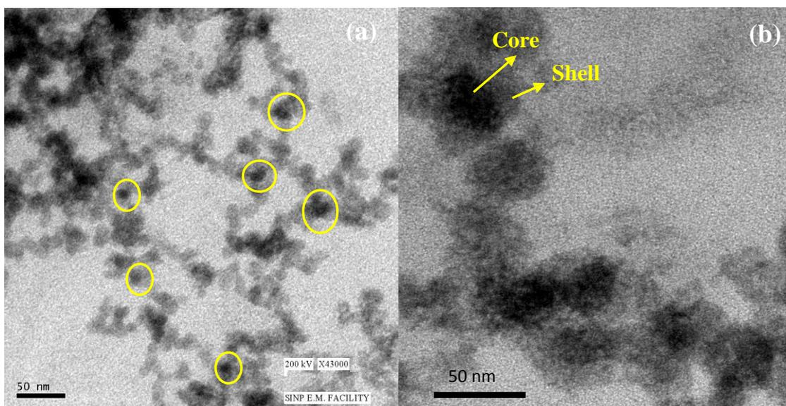
**Figure 8.3** (a) TEM and (b) Higher magnification (X71,000) TEM micrograph obtained for  $Gd_2O_3/NiO$  CSNPs
